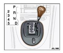
The switch also provides an output signal NEUTRAL, when the gear position neutral is selected. It monitors the mode switch status and provides an output to switch the mode switch status LED in accordance with the mode switch operation strategy.
