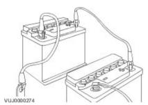
WARNING: Make sure that the ends of the jump leads do not touch each other or ground against the vehicle body at any time while the leads are attached to the battery. A fully charged battery, if shorted through jump leads, can discharge at a rate well above 1000 amps causing violent arcing and very rapid heating of the jump leads and terminals, and can even cause the battery to explode.
