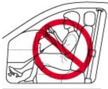
Wrong Unbelted and too close
