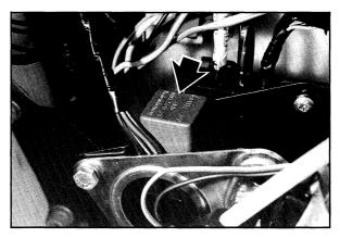
Location: On left motor/winch assembly. Function: Provides an ECM signal when reverse is selected to prevent system
