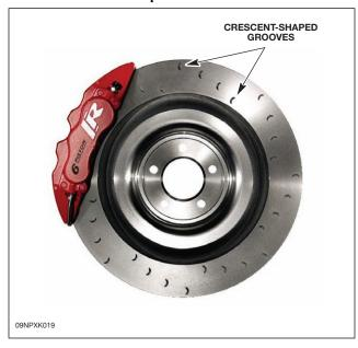
Front brakes use a 40cm (15.75 in.) brake disc and a 6-piston caliper. Rear brakes use a 35cm (13.78 in.) brake disc and a 4-piston caliper.
