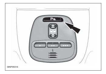
Pressing the switch turns both the front and rear parking aid on or off. The integral switch warning indicator light will come on when the system is turned on, or if a fault is detected in the system.
