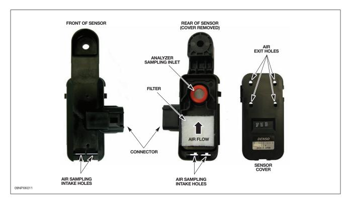
The pollution sensor is powered by an ignition-controlled voltage feed from the central junction box (CJB) and provides separate input signals for hydrocarbon and oxidized gas levels to the ATCM.
