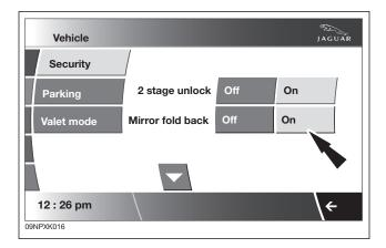
Automatic operation is synchronized with the exterior locking and unlocking of the vehicle (it does not work with interior locking and drive-away locking). If automatic operation is selected, the door mirrors fold when the vehicle is locked and unfold when the vehicle is unlocked.
