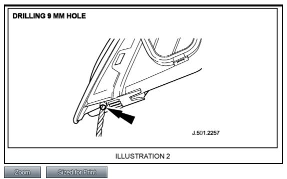
4. Carefully drill a 9 mm diameter hole upwards into headlamp using the stub pipe as a guide (Illustration 2).
