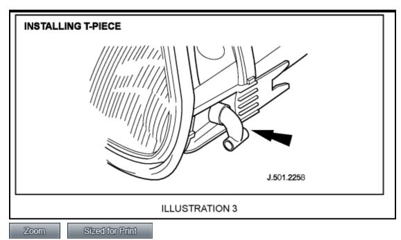
6. Install and align T-piece to stub pipe (Illustration 3).
