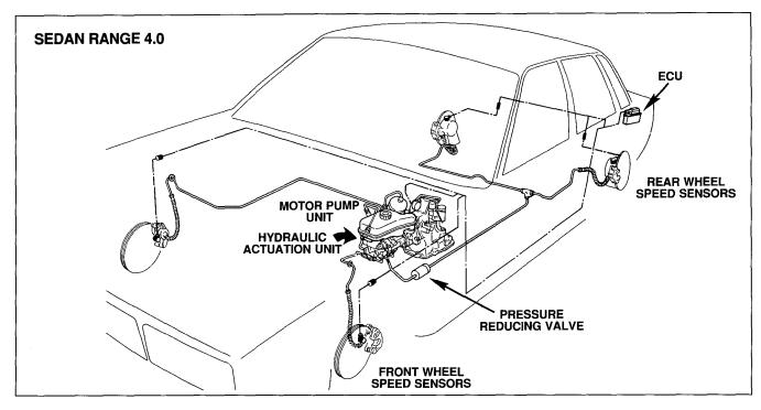
The TEVES brake system combines normal system operation, power boost and anti-lock braking. The system uses an independent electrically-driven motor pump unit to provide both boost pressure and brake application pressure. A common operating fluid, DOT 4 BRAKE FLUID, is used for both power boost and brake application.
