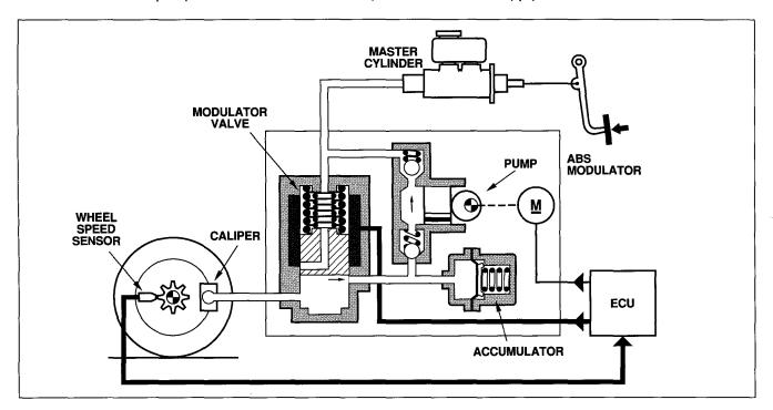
**Third Stage: Pressure Increase (Normal Brake Operation)** The solenoid value is positioned to allow normal hydraulic flow to and from the brake caliper(s).
