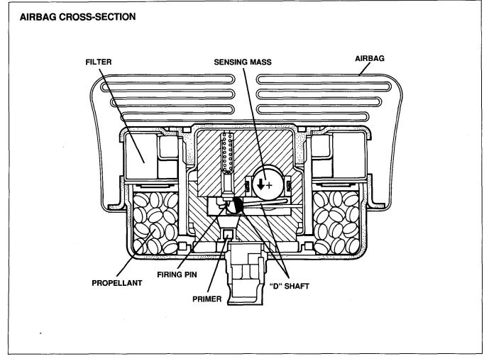
**Crash sensing** In the event of a frontal impact, the vehicle body structure will deform, absorbing the energy of the impact. The crash pulse is transmitted to the steering column, then to the steering wheel, then to the inflator / sensor.
