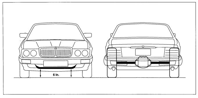
With the vehicle resting on sliding wheel plates, tool JD 145 is installed at the rear with the large hook located around the drive shaft. After careful compression of the rear suspension, the small or upper hook is then attached to the top of the rebound stop. Next, tool JD 133 is used to compress the front suspension until the measurement between the wheel plates and the bottom of the subframe is 6 in. on both sides.
