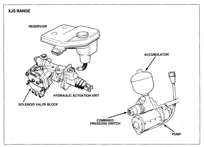
In the XJS, the motor pump unit is located separately on the right side of the front bulkhead. The reservoir and the hydraulic actuation unit are integrated on the brake pedal and accelerator housing. The motor pump unit contains the hydraulic pump, motor, accumulator and combined pressure switch. The hydraulic actuator incorporates many components including the solenoid valve block.
