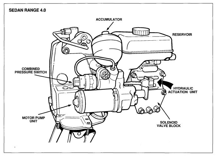
In the Sedan Range, the motor pump unit, reservoir and hydraulic actuation unit are integrated on the brake pedal and accelerator housing. The motor pump unit contains the hydraulic pump, motor, accumulator and combined pressure switch. The hydraulic actuator incorporates many components including the solenoid valve block.
