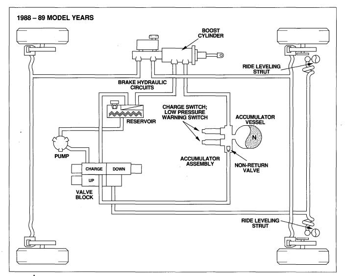
**CAUTION:** THE RIDE LEVELING SYSTEM WILL ALLOW THE VEHICLE TO BE OVER-LOADED WITHOUT A PERCEPTIBLE CHANGE IN TRIM HEIGHT. ENSURE THAT THE SPECIFIED VEHICLE GROSS WEIGHT IS NOT EXCEEDED WHEN LOADING.
