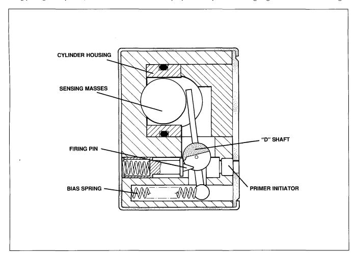
If the specified impact occurs, two spherical "sensing masses" move forward against levers which rotate the "D" shafts. Two bias springs return the "D" shafts to their seated positions if an impact is insufficient to fully trigger the sensing masses. The "D" shafts can be prevented from rotating by carrying out a disarming procedure so that service and maintenance work to be safely conducted.
