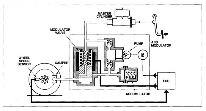
**Second Stage: Pressure Reduce** If the wheel continues to decelerate, the solenoid valve return port is opened, reducing the hydraulic pressure to the caliper and allowing the wheel to accelerate. When the return port is opened, the ECU activates the pump to recirculate the returned hydraulic fluid to the supply side of the accumulator.
