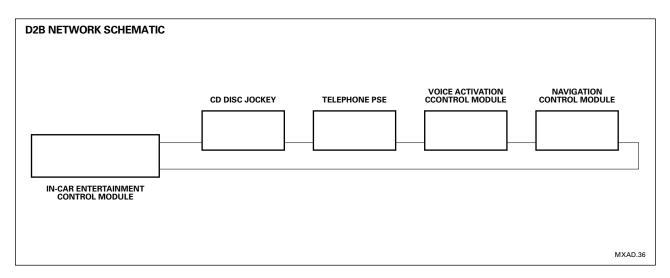
The wake up command is a separate, hard wired electrical pulse sent from the ICE to the other modules. The ICE sends this pulse in response to the key being turned to the accessory position. This turning triggers the modules to look for the first light signal sent out by the ICE. At the end of this initialization procedure, the modules are ready for full network operation. If any part of this initialization fails, DTCs will be logged.
