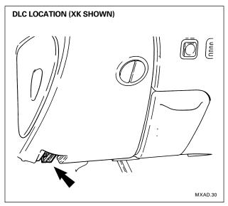
Both the CAN and SCP busses are directly connected to the DLC. WDS contains hardware and software that allows it to function as a "node," an additional module added to networks. The software and hardware supports direct communications between WDS and the networks for diagnostics and module programming. In addition, WDS communicates via the DLC with nonmultiplexed modules using a Serial Data Link (ISO 9141).
