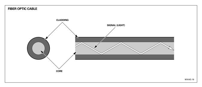
Instead of copper cables, this system uses fiber optic cables made of plastic.
