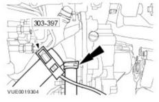
$\ensuremath{\mathbf{27}}$  . Disconnect the turbocharger vacuum hose.
