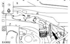
55 . Detach the engine wiring harness earth lead.
