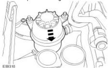
23 . Install the power steering fluid reservoir retaining nuts.
