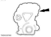
78 . Using the special tool 303-682, install the engine front cover.
