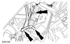
4 . Disconnect the vacuum solenoid valves electrical connectors.
