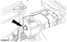
${\bf 35}$  . Disconnect the glow plug harness electrical connector.
