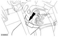
42 . Remove the exhaust manifold to E.G.R valve tube. For additional information, refer to
