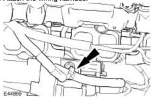
29 . Connect the fuel metering valve and fuel temperature sensor electrical connectors.
