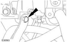
$\boldsymbol{8}$  . Detach the engine wiring harness from the intake manifold rear retaining bracket.
