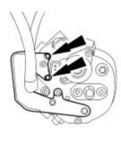
4 . Install the fuel injection pump shield retaining bolt.
