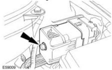
40 . Disconnect the glow plug harness electrical connector.
