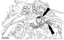
30 . Remove the engine wiring harness.
