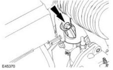
3 . Install the EGR cooler to EGR valve tube support bracket lower retaining bolts.
