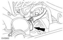
8 . Remove the generator upper retaining bolt.
