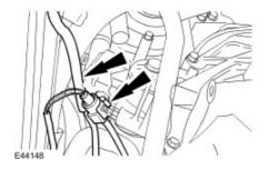
8 . Remove the wiring harness support bracket.
