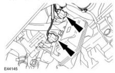
${\bf 5}$  . Detach the wiring harness from the vacuum solenoids and vacuum reservoir mount bracket.
