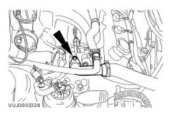
74 . Connect the spring lock coupling.
