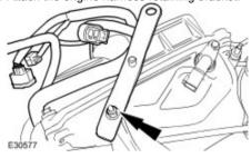
101 . Disconnect the right-hand camshaft position sensor.
