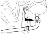
28 . Disconnect the air temperature sensor electrical connector.
