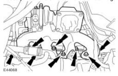
8 . Install the exhaust manifold gasket retaining studs.
