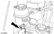
14 . Remove the engine mount damper.
