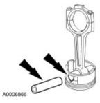
2 . Install the retaining clips.
