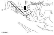
101 . Remove the transmission upper retaining bolts.
