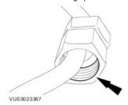
CAUTION: Do not allow the unions to hit the olive ends of the high pressure fuel supply line as this may damage the ends of the line and allow foreign matter to enter the fuel injection system.
