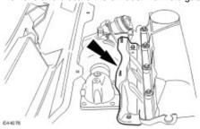
26 . Remove the turbocharger.
