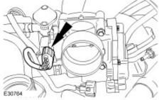
123 . Connect the throttle motor electrical connector.
