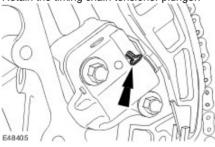
17 . Remove the left-hand timing chain tensioner.
