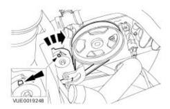
42 . Remove the power assisted steering pump bracket retaining bolts.
