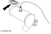
21 . Install new catalytic converter retaining studs.
