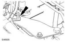
$\boldsymbol{8}$  . Connect the positive crankcase ventilation (PCV) hose to the valve cover.
