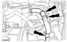
53 . Connect the power assisted steering hose.
