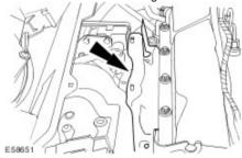
3 . Attach the turbocharger to the cylinder head.
