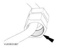
43. Remove the blanking plugs from the fuel injection pump and fuel injection supply manifold threaded ports.
