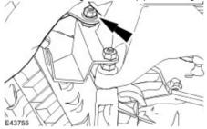
86 . Detach the reverse lamp switch wiring harness retaining clip.
