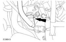
51 . Disconnect the knock sensor (KS) electrical connector.
