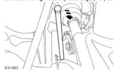
74 . Connect the air temperature sensor electrical connector.
