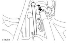
76 . Connect the air temperature sensor electrical connector.
