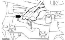
12 . Remove the vacuum solenoid mount bracket assembly.
