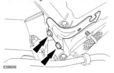
72 . Install the engine rear lifting eye.
