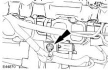
5 . Clean the fuel pump, high pressure fuel supply line and surrounding areas. For additional information, refer to Fuel Injection Component Cleaning
