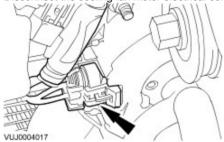
4 . Disconnect the cooling fan module electrical connectors.
