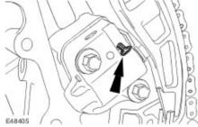
9 . Remove the right-hand timing chain tensioner.
