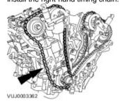
51 . Install the right-hand timing chain outer guide.
