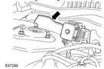
${\bf 55}$  . Attach the engine wiring harness retaining clip.
