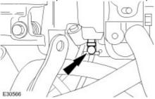
114 . Attach the intake manifold rear retaining bracket.
