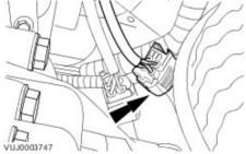
87 . Disconnect the right-hand heated oxygen sensor (HO2S) electrical connector.
