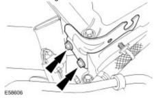
76 . Install the engine rear lifting eye.
