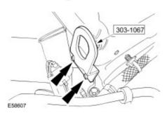
$\boldsymbol{8}$  . Using the special tool, support the engine and transmission assembly.
