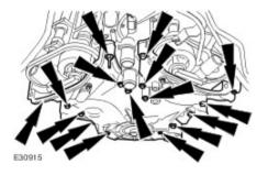
58 . Remove the crankshaft position (CKP) sensor pulse wheel.
