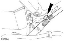
${\bf 5}$  . Detach the electrical connector from the engine cover mounting bracket.
