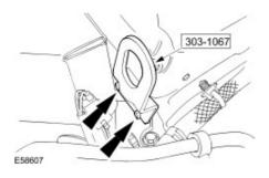
31 . Install the engine cover rear mount bracket.
