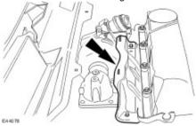
6 . Attach the turbocharger to the cylinder head.
