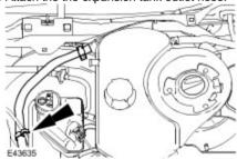
64 . Connect the expansion tank outlet hose.
