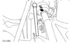
30 . Detach the charge air cooler outlet hose from the charge air cooler.
