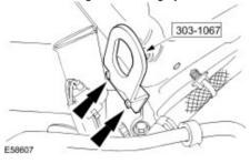
26 . Install the engine cover rear mount bracket.
