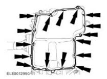
Tighten the bolts in the sequence shown in two stages.
