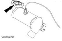
26 . Install new catalytic converter retaining studs.
