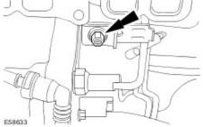
10 . Clean the fuel injection pump, high-pressure fuel supply line and surrounding areas. For additional information, refer to <a href="Fuel Injection Component Cleaning">Fuel Injection Component Cleaning</a>
