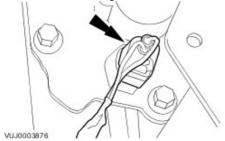
73 . Install the clutch master cylinder to clutch slave cylinder high pressure pipe support bracket.
