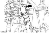
154 . Install the turbo outlet pipe retaining bolt.
