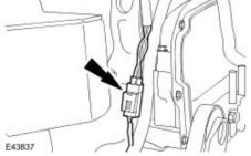
9 . Remove the wiring harness.
