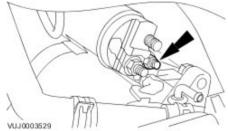
12 . Remove the starter motor rear retaining bolt.
