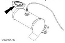
92 . Using the special tool, detach the transfer case link shaft.
