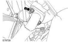
${\bf 9}$  . Remove the EGR valve tube to EGR valve retaining studs.
