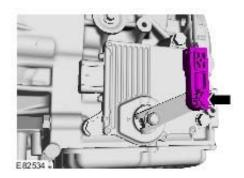
Install the transmission control module (TCM).
