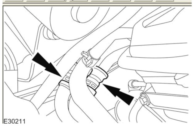
Disconnect the auxillary coolant flow pump electrical connector.
