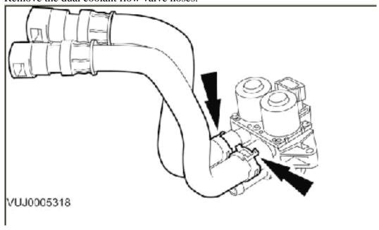
To install, reverse the removal procedure. Tighten to 10 Nm.
