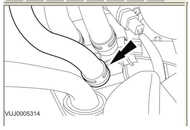
For vehicles fitted with 4.2L engine Remove the radiator upper hose.
