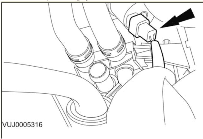
Remove the dual coolant flow valve: 1.) Remove the retaining bolt. 2.) Remove the dual coolant flow valve.
