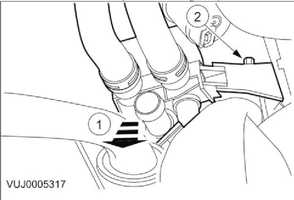
Remove the dual coolant flow valve hoses.
