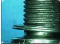
Example of 10mm thread spark plug broken during installation due to the use of anti-seize leading to over-tightening. (Note that plug gasket has been completely compressed, anti-seize can be seen on threads, and the break is in the direction of tightening).
