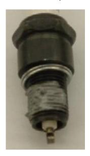
Example of spark plugs that do not have metal shell plating
