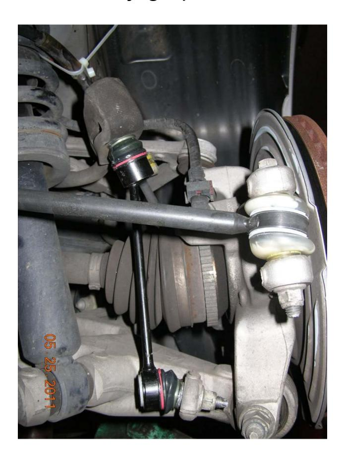
**Torques:** Inner Nut 100Nm (74 ft. lbs.) Outer Nut 55Nm (41 ft. lbs.)
