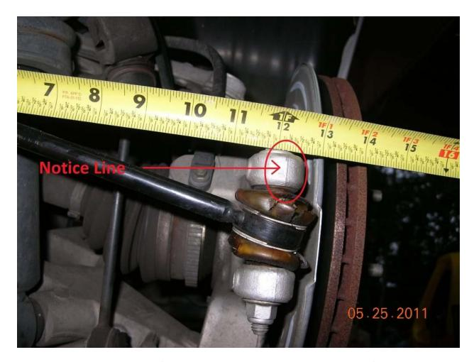
Next using the 18mm box wrench (here is where a ratcheting wrench works the best) and the 8mm box end, remove the inner tie rod nut. Then move to outer tie rod end using the 13mm wrench and 15mm socket. Pull bolt out and remove tie rod assembly.
