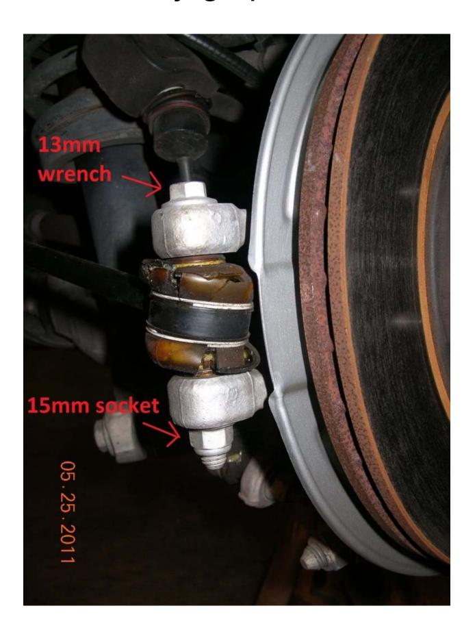
Start inner tie rod nut, align outer tie rod with phillips screw driver, push in and insert bolt.
