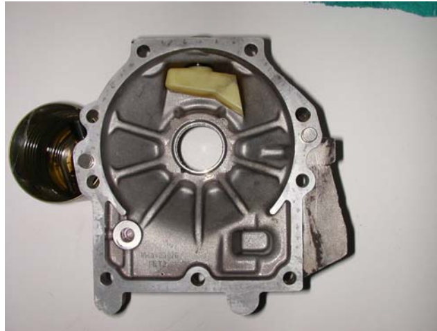
Fig. 15 Internal view of extension case
