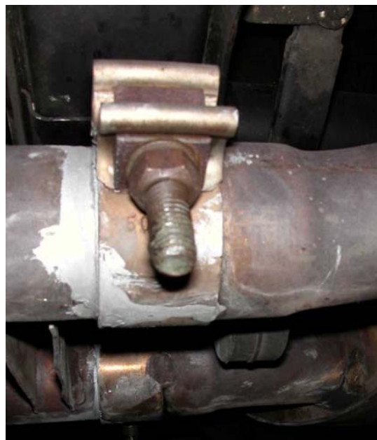
Fig. 5 Side view of rear-catalyst outlet pipes and clamps
