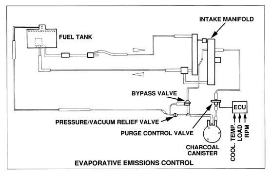
The charcoal canister, purge control valve, bypass valve, and pressure/ vacuum relief valve are located ahead of the left front wheel arch.
