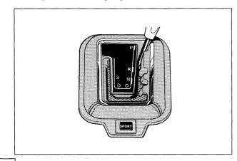
**NORMAL mode** This strategy is designed for everyday use. With "D" selected, torque converter lock-up occurs in fourth gear only; with "3" selected, lock-up occurs in third gear.
