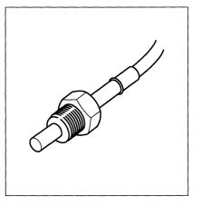
**Location** In the EGR adaptor under the intake manifold.
