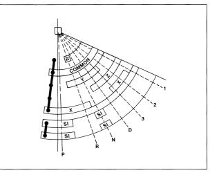
When the driver selects a gear, the selector bar moves across the quadrant to a pre-determined position to contact the copper segment(s). The copper segments are set out in seven bands across the quadrant with each band providing an output or combinations of outputs to the decoder module. Outputs are in the form of a three-digit XYZ code. Three quadrant segments are used for the three-digit code; the remaining four segments are used for REVERSE, ground [common], and start inhibit [SI].
