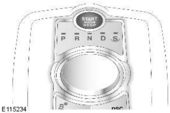
The Jaguardrive selector is a rotary selector installed in the top of the JaguarDrive selector module. The JaguarDrive selector module is located in the floor console and controls the vehicle optimization functions on the vehicle. For additional information, refer to: Ride and Handling Optimization (204-06 Ride and Handling Optimization, Description and Operation).
