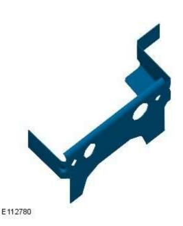
NOTE: The hood latch panel mounting bracket is manufactured from mild steel.
