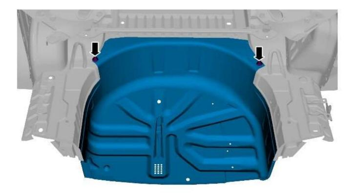
13. ONOTE: Remove the sealer to expose the spot welds.Drill out the spot welds.
