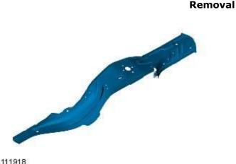
1. NOTE: The rear side member closing panel section is manufactured from High Strength Low Alloy Steel, 350MPa, (HSLA350).
