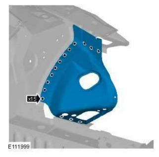
4. NOTE: Spot welds must be installed 5mm away from the originals and in the same quantities, whenever this is possible. Where this is not possible, spot welds should be installed adjacent to the original.
