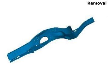
1. NOTE: The rear side member section is manufactured from High Strength Low Alloy Steel, 350MPa, (HSLA350).
