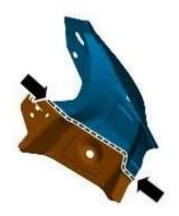
12. **O**NOTE: It may be necessary to remove or bend the safety belt mounting part of the template to aid alignment. Retain the template as this will be used to form a backing plate.
