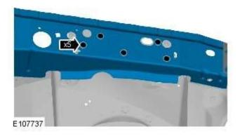
12. NOTE: If the fender mounting plate is undamaged it can be reused by releasing it from the fender apron panel, leaving it attached to the suspension top mount. Drill out from underneath to allow spot welds to be used in installation.
