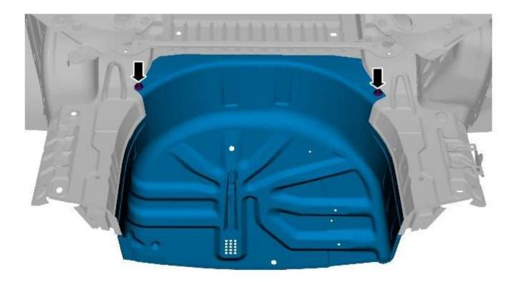
10. NOTE: Spot welds must be installed 5mm away from the originals and in the same quantities, whenever this is possible. Where this is not possible, spot welds should be installed adjacent to the original.
