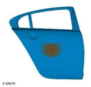
1. NOTE: The rear door is manufactured from mild steel, it contains a side impact reinforcement manufactured from boron steel.
