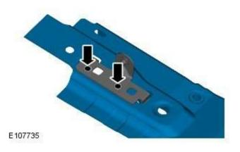
10. NOTE: If the hood strut mounting bracket is to be replaced, it is not necessary to remove it.
