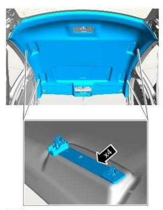
20. CAUTION: Note the fitted position of the component prior to removal.
