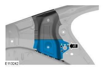
15. **C**NOTE: The right-hand panel is illustrated, the left-hand is similar although there are additional spot welds to drill out.
