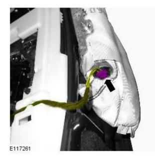
WARNING: Do not probe supplemental restraint system (SRS) electrical connectors. 18.
