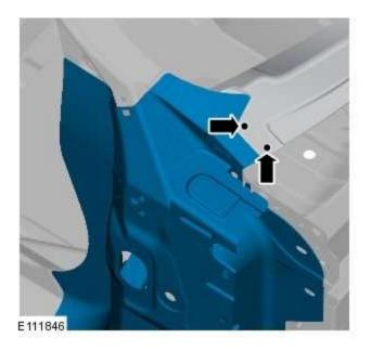
2. With the new panel in position, mark the position of MAG plug welds as indicated.
