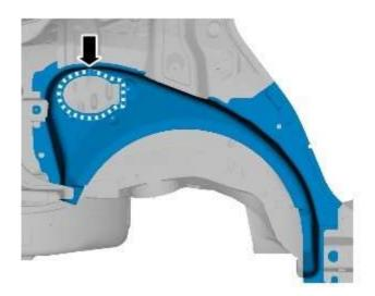
34. If the right-hand rear wheelhouse outer is being repaired, prepare the NVH component at the fuel filler aperture, apply sealer adhesive, and install as indicated.
