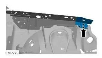
6. NOTE: Spot welds must be installed 5mm away from the originals and in the same quantities, whenever this is possible. Where this is not possible, spot welds should be installed adjacent to the original.
