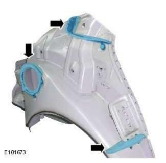
Separate the joints and remove the old panel, also releasing the <u>NVH</u> components.
