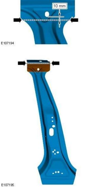
NOTE: Dress the panel joint surfaces of the template to ensure a good fit. 2.
