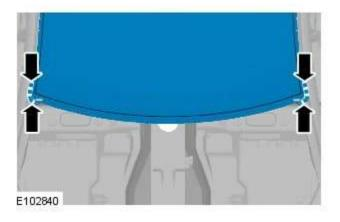
10. Make sure the external areas around the MIG brazed slots are sealed as part of the paint preparation process as this cannot be performed satisfactorily during panel replacement.
