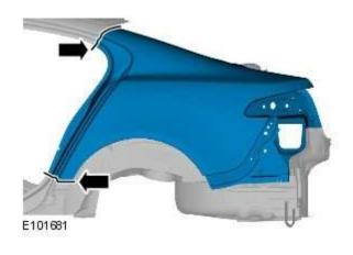
16. MAG weld the butt joints.
