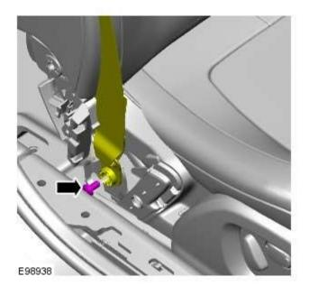
4. NOTE: Right-hand shown, left-hand similar. Release the safety belt lower anchor from the front seat.
