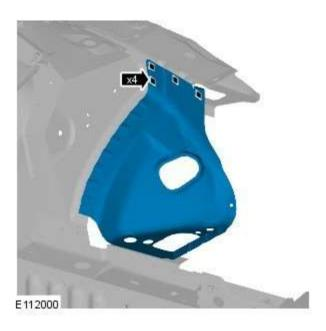
5. NOTE: If adjacent panels are being repaired and access allows, spot welds should be installed where possible.
