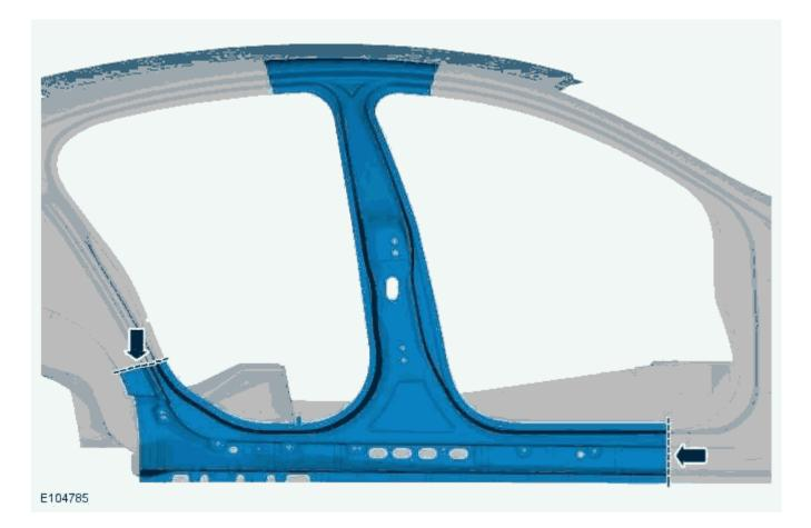
35. Drill out the spot welds.
