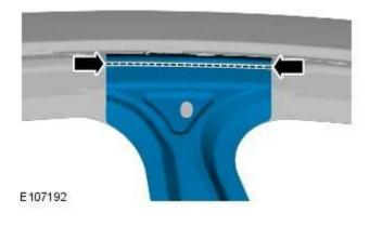
NOTE: A drill bit suitable for drilling boron should be used on the 6. boron spot welds.
