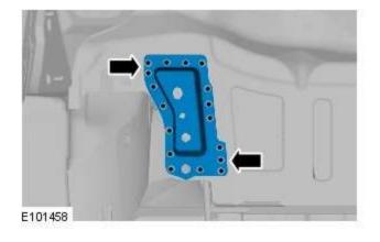
4. NOTE: Spot welds must be installed 5mm away from the originals and in the same quantities, whenever this is possible. Where this is not possible, spot welds should be installed adjacent to the original. Where there is adhesive in the original joint, spot welds should be installed through the original.
