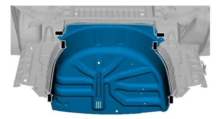
14. NOTE: Retain the old panel for reference to the weld stud location points.
