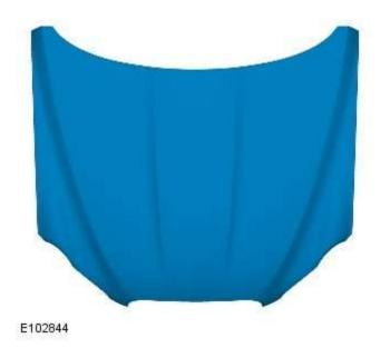
NOTE: The hood is manufactured from aluminium. The hood is serviced as a separate bolt-on panel.
