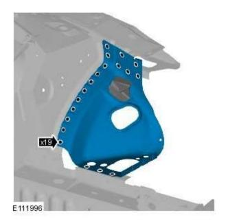
7. NOTE: If the left-hand front wheelhouse section is to be repaired, retain the old panel if the air cleaner mounting bracket is to be reused.
