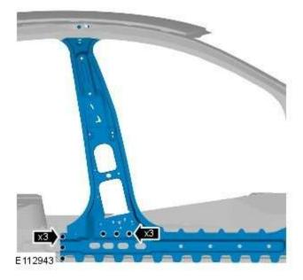
7. Drill out the spot welds.
