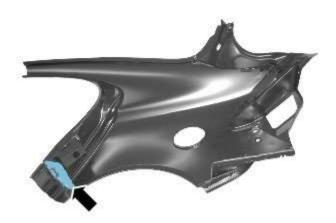
35. ANOTE: The NVH component at the striker reinforcement panel should be installed with the new quarter panel, sealer adhesive should be applied as the new quarter panel is installed.
