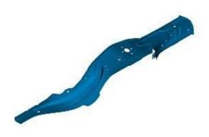
NOTE: The rear side member closing panel section is manufactured from High Strength Low Alloy Steel, 350MPa,
