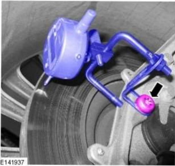
12. Remove DTI and install the bait. 90 Nm.
