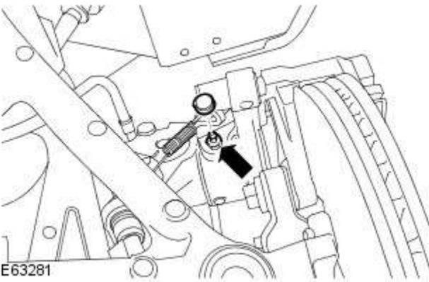
7. Loosen the bleed screw by one-half to three-quarters of a turn.
