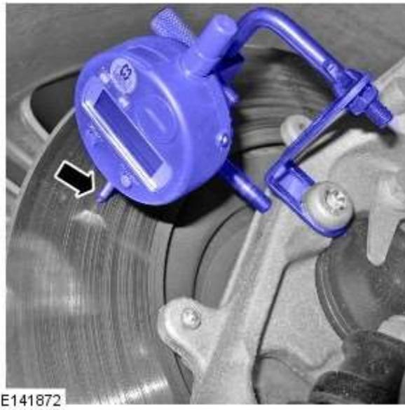
6. Position the DTI probe in the centre of the disc.
