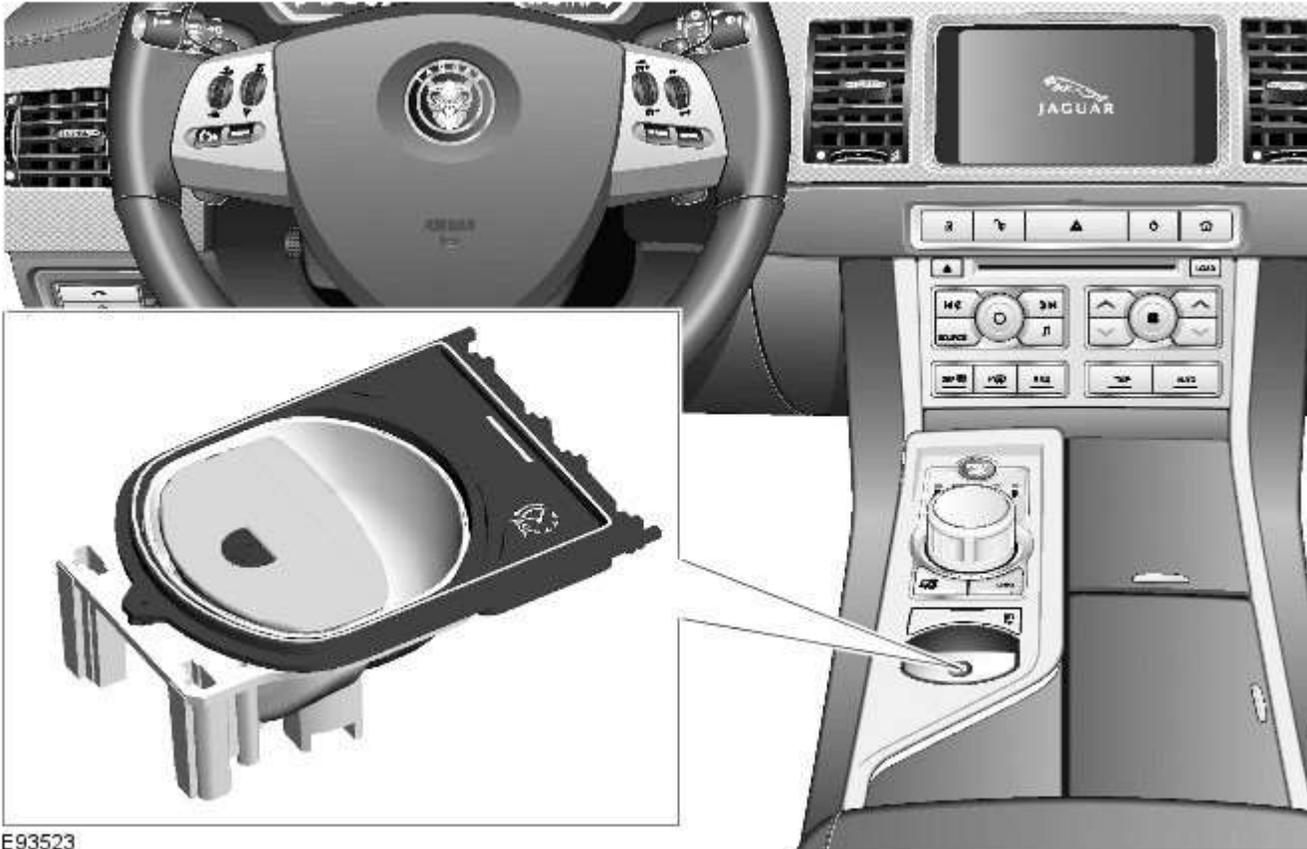
The parking brake switch is mounted in the floor console, rearward of the rotary gear selector. The switch has 3 states:
