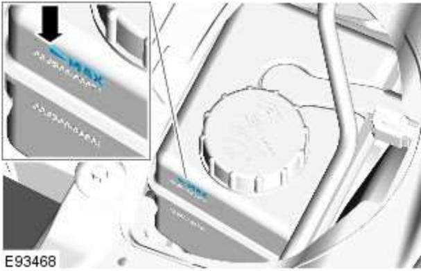
Fill the brake fluid reservoir to the MAX mark.
