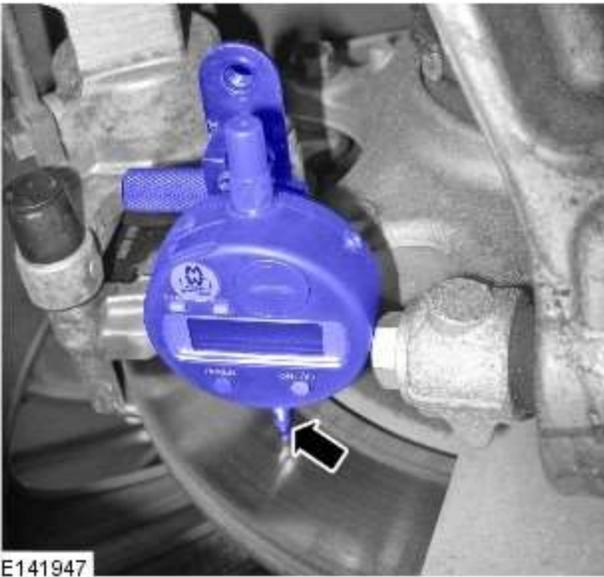
8. Position the DTI probe 5 mm from the inner edge of the disc.
