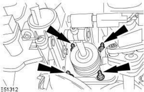
5. Remove the brake booster retaining nuts.
