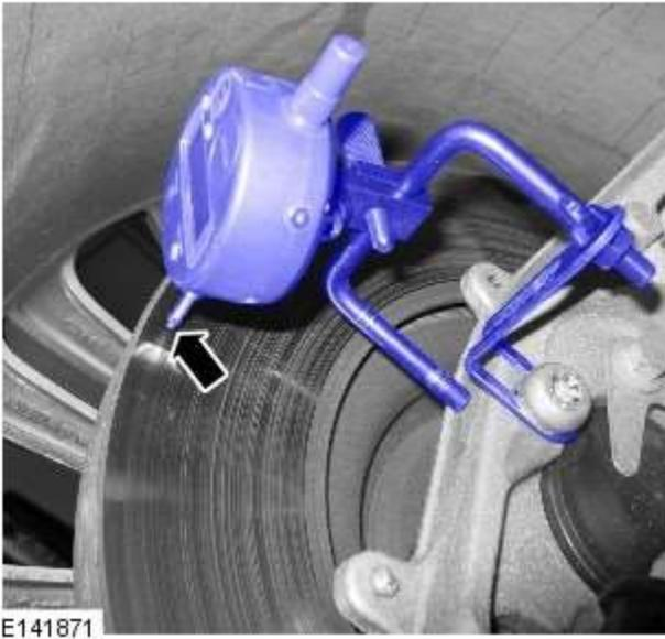
5. Position the DTI probe 5 mm from the outer edge of the disc.
