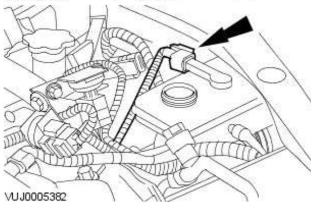
2. Disconnect the brake fluid level electrical connector.
