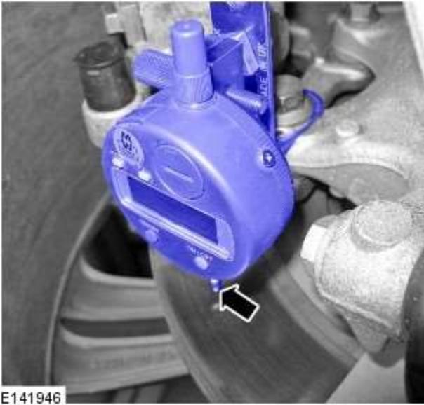
7. Position the DTI probe in the centre of the disc.
