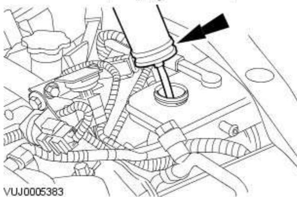
3. Using a suitable suction device drain the brake fluid reservoir.
