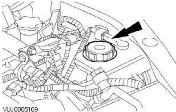
1. Remove the brake fluid reservoir cap.
