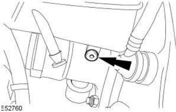
4. Remove the brake fluid reservoir.
