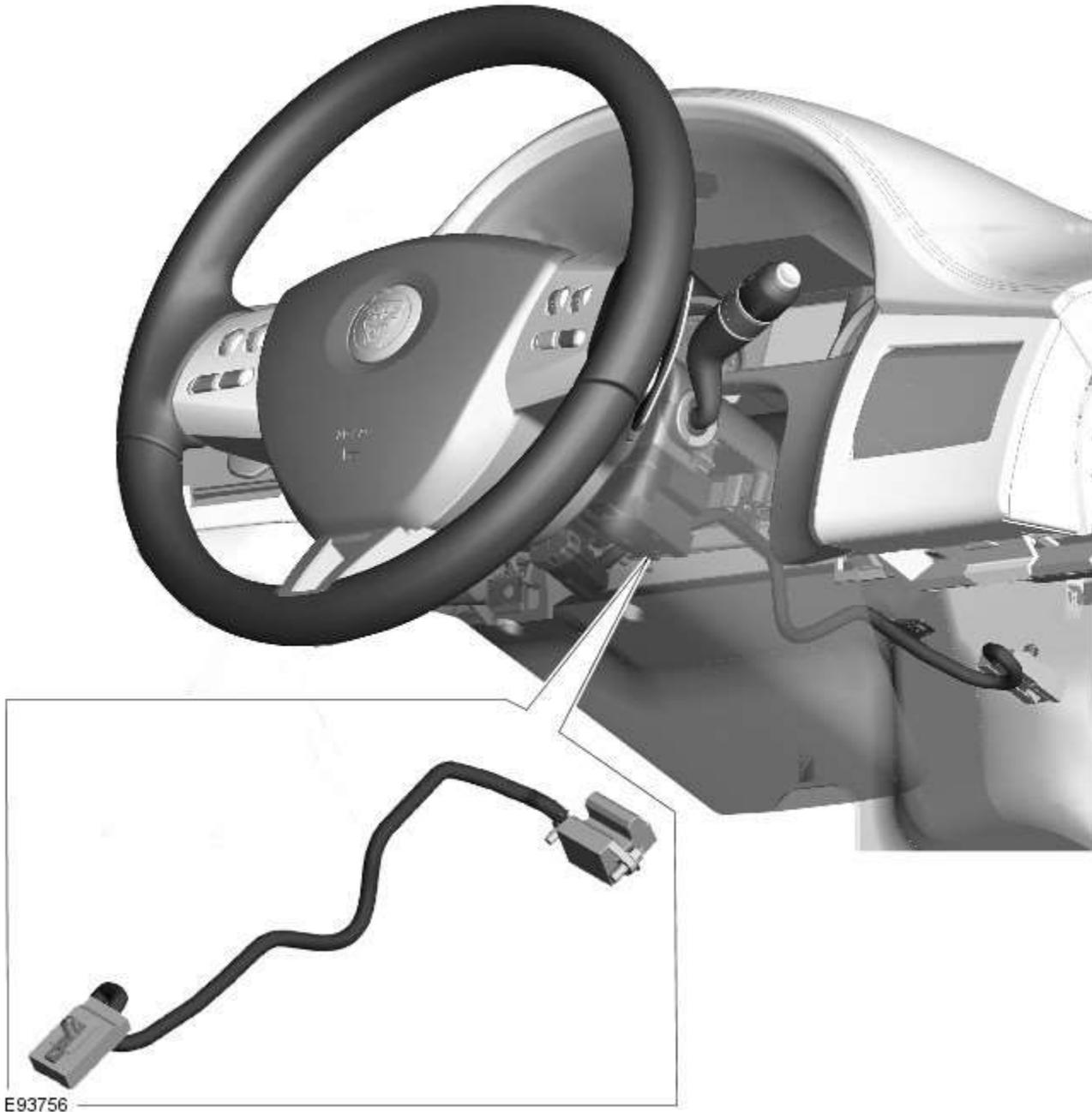
The steering angle sensor measures the steering wheel angle and the rate of change of the steering wheel angle. These measurements are received by the [ABS](#) module and broadcast on the high speed [CAN](#) bus for use by other systems.
