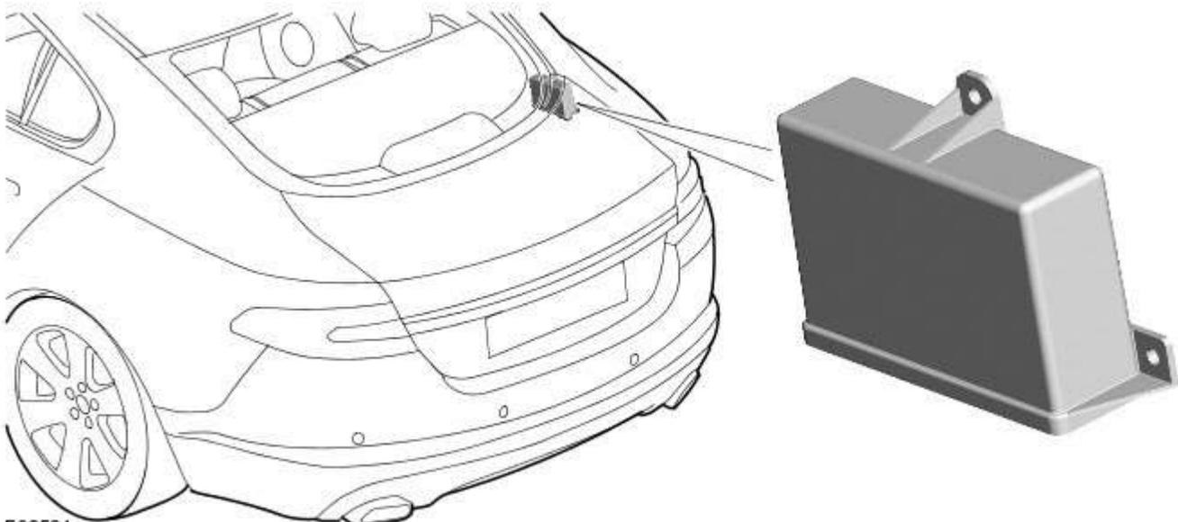
The EPB module is mounted in the luggage compartment on the **RH (right-hand)** side quarter panel and is connected to the vehicles electrical wiring by two multiplugs. The EPB module is also connected to the high speed **CAN** bus, allowing it to communicate with other vehicle systems.
