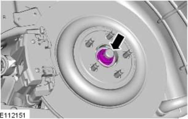
3. With assistance, remove the halfshaft retaining nut, and retain it for the install procedure.
