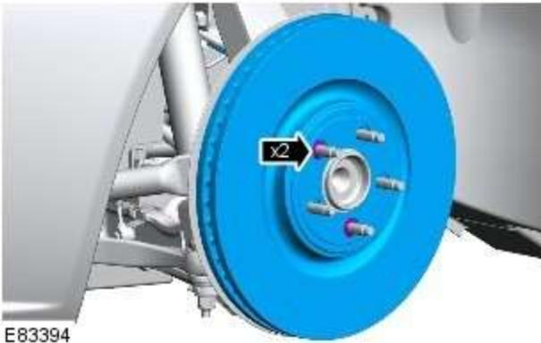
5. Remove the rear brake disc.
