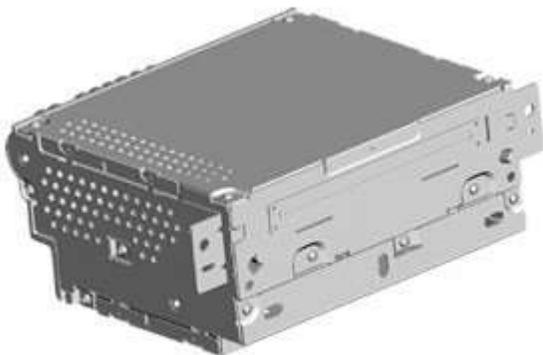
The IAM is located in the center console behind the ICP faceplate, and combines the radio tuner and [CD](#) player. The head unit controls which of the two sources is routed to the speakers. All tuner versions have AM/FM reception. Each audio system features auto-store, with a press and hold function to store selected channels as pre-sets. The standard search facility finds the nine strongest channels currently available, while search and manual tuning allow channels to be stored as above.
