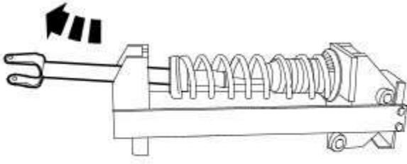
15. Remove the front shock absorber.
