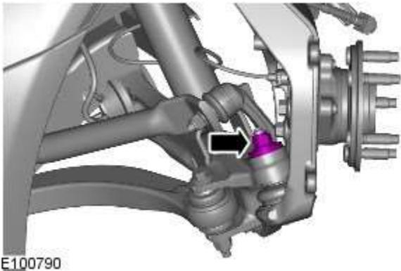
1. NOTE: Use an additional wrench to prevent the ball joint rotating.
