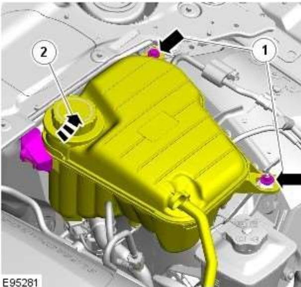
6. Secure the coolant expansion tank.
