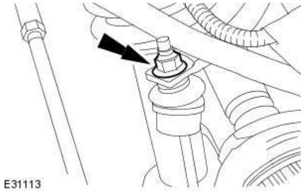
19. Remove the stabilizer bar link nuts.
