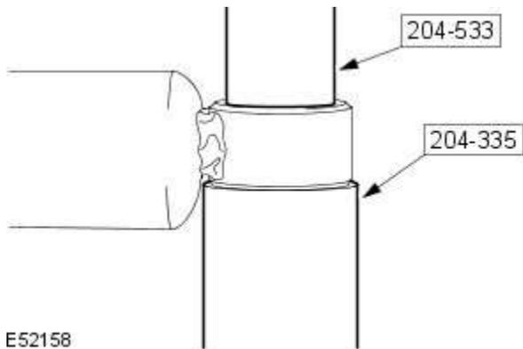
5. Using the special tools, carefully remove the bushing from the shock absorber.
