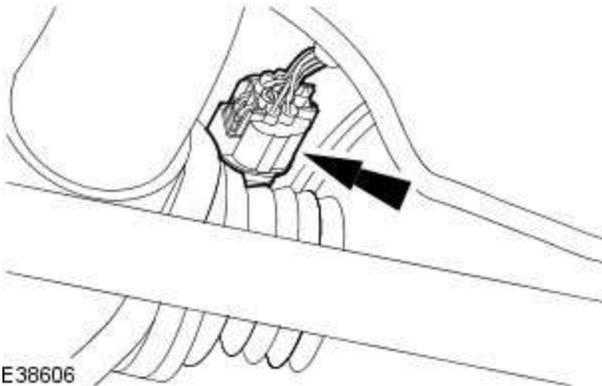
9. Disconnect the electronic parking brake actuator electrical connector.
