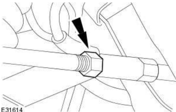
8. **NOTE:** LH illustration shown, RH is similar. To adjust, loosen the toe link locknuts.
