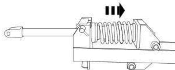
14. Carefully release the spring tension.
