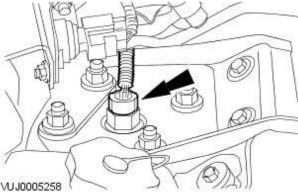
4. Connect the front shock absorber electrical connector.
