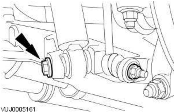
3. Release the shock absorber and spring assembly from the lower arm.
