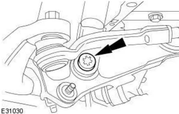
9. Connect the front shock absorber and spring assembly to the lower arm.
