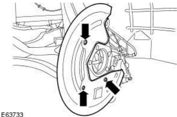
4. Install the brake disc shield.
