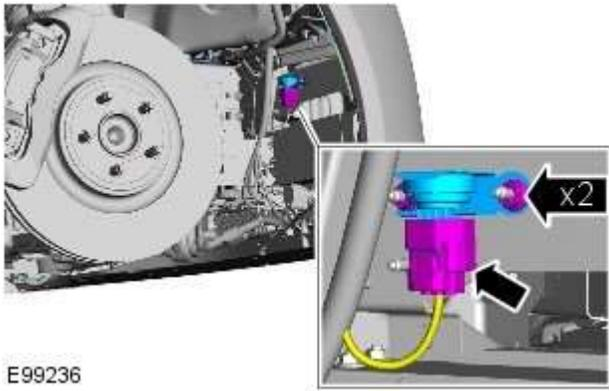
3. **CAUTION:** The accelerometer is an extremely delicate component and can easily be rendered unserviceable. Never use an accelerometer which has been dropped or subjected to mistreatment of any type.
