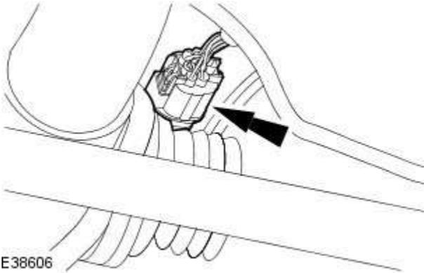
15. Connect the wheel speed sensor electrical connector.
