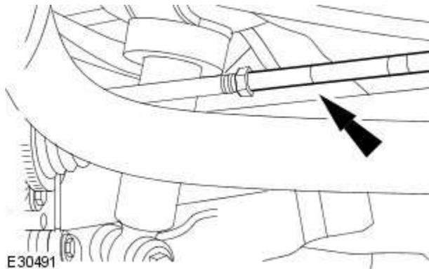
4. Rotate the toe link to adjust the toe settings.
