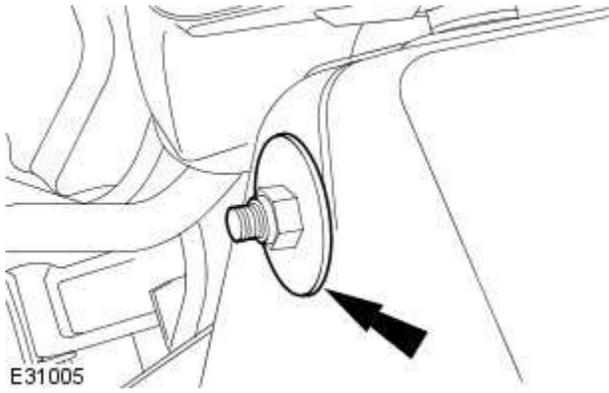
5. CAUTION: The final tightening of the suspension components must be carried out with the vehicle on its wheels.
