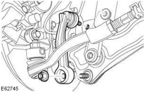
3. **NOTE:** Use an additional wrench to prevent the ball joint rotating.
