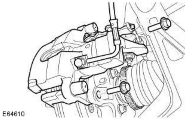
17. Connect the brake hose to the brake caliper.
