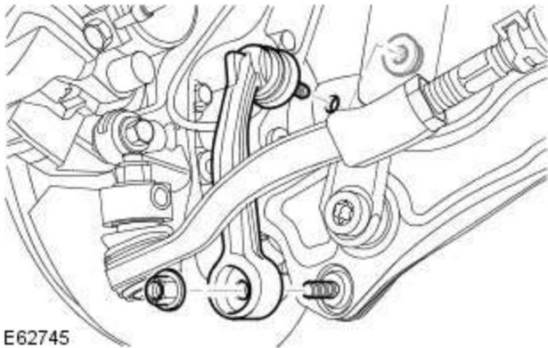
1. **NOTE:** Use an additional wrench to prevent the ball joint rotating.
