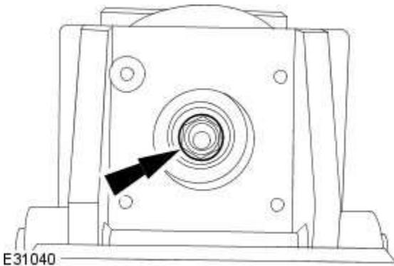
13. Remove the front shock absorber retaining nut
