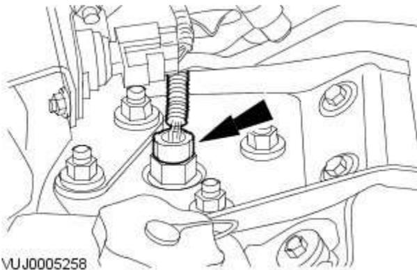
9. Disconnect the front shock absorber electrical connector.
