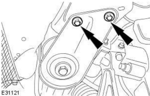
9. Tighten the rear subframe reinforcement plate retaining bolts.
