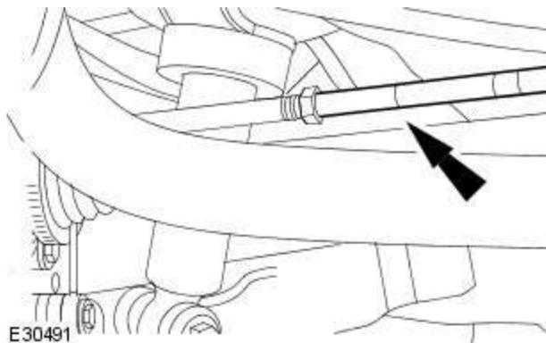
5. Tighten the lock nut.
