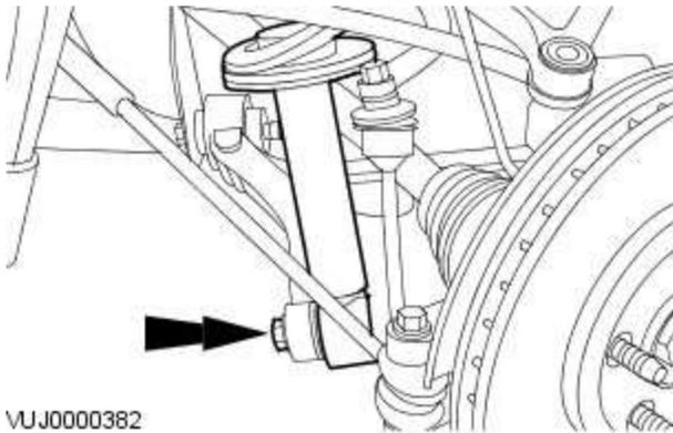
4. Install the shock absorber and spring assembly.
