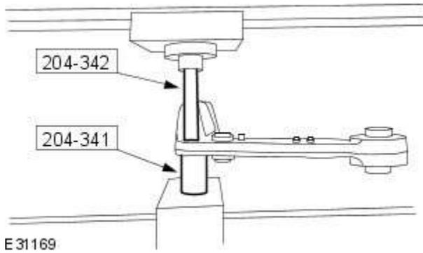
3. Using the special tools, remove and discard the stabilizer bar link bushing.
