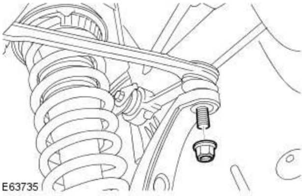
2. NOTE: Use an additional wrench to prevent the ball joint rotating.
