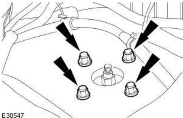
6. Install the shock absorber and spring assembly top mount nuts.
