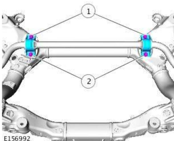
28. During installation tighten the bolts in the following sequence.
