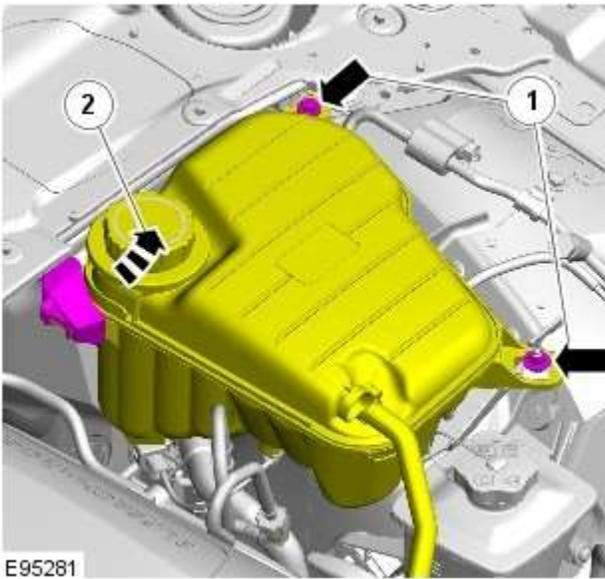
8. Release the coolant expansion tank for access.
