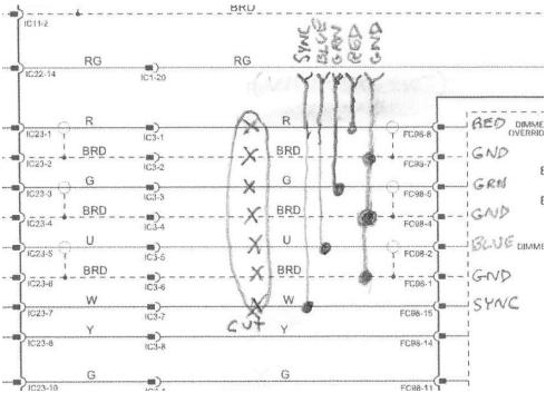
Also, before connecting the converter, definitely follow the advice in the instructions and test mate the two molex connectors that are spliced in the circuit to make sure your splices are done property.
