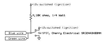
The three positions of the switch are then video 1 (center to +12), original nav. video (center off) and video 2 (center to ground).
