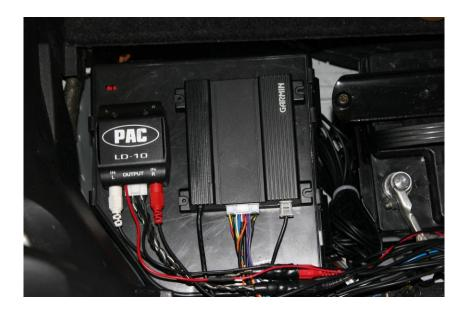
A convenient source of power in the trunk is the trunk accessory connector, which is an unused three pin connector adjacent to the battery which provides Ignition switch power, battery +12v and ground. Be sure to check whether trunk fuse box relay number 6 and fuse number 11 are present...you may need to add them. The relay is a standard automotive single pole type available from any auto parts store.
