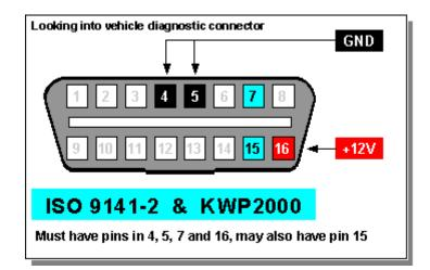
The same wake-up information is also carried on pin 7, the main data signal. All you have to do is connect pin 15 to pin 7 on the HKS CAMP 2 OBDII harness to make it work. The problem is the HKS CAMP OBDII 2 connector does not contain pin 15.
