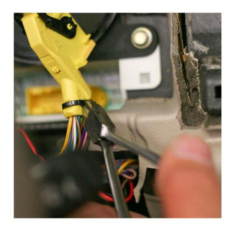
14. On each of the connectors, pry off the hood retainer gently with a pair of pliers.
