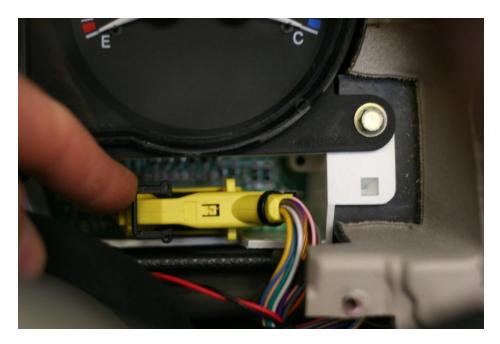
20. Tuck the black and red wires under the speedometer white plastic shell:
