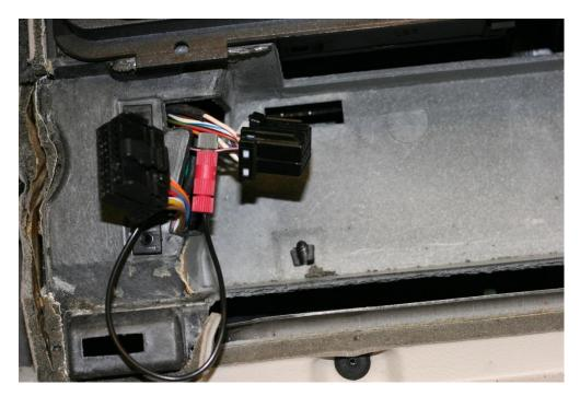
11. Locate the two main instrument panel connectors. One is yellow and the other is black.
