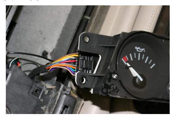
22. Using the screws removed from the navigation monitor, fasten the new gauge cluster to the dash.
