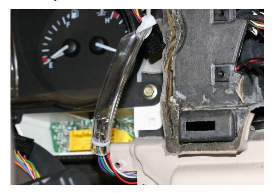
8. Clip the tie-wrap off of the clear tubing on the pulling tool and withdraw the tool from the wires. You may need to stagger the terminals in the clear tube to get them out without excessive force.
