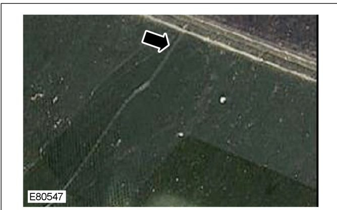
13. Crack along roof line.
