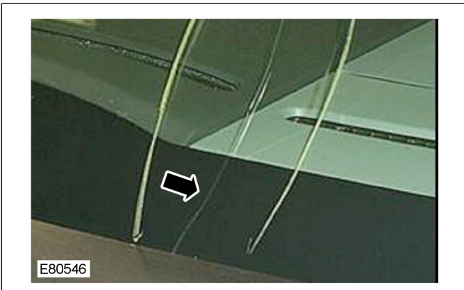
13. Crack along roof line.
