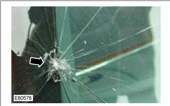
11. High impact resulting in many cracks.
