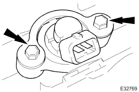
5. Remove bolts which secure fuel injector clamp plate to inlet manifold.
