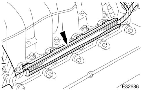
4. Disconnect bank 1 or 2 injector connectors and reposition harness to allow access to injectors.
