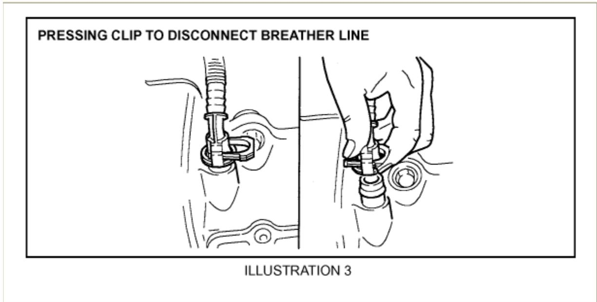
6. Depress the retaining clip (Illustration 3) of the connector of the part-load breather line, allowing the line connector to be disconnected from the breather stub on the left camshaft cover.
