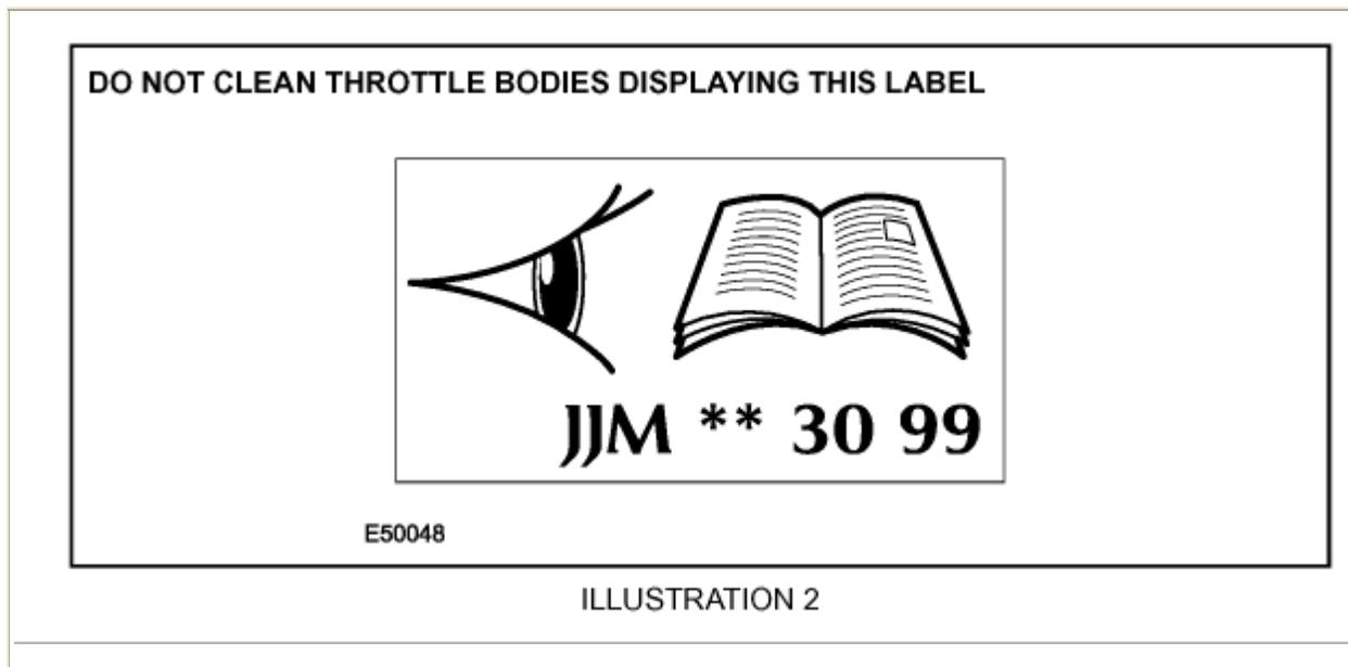
**\*Caution :** If the [throttle body](#) displays the label shown in Illustration 2, do not clean the throttle body bore and butterfly valve as damage to the vehicle can result.\*
