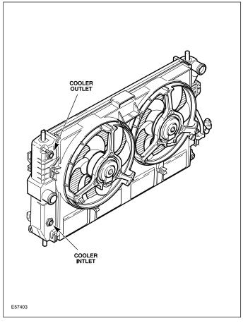
Separate Oil Cooler (Air to Liquid)
