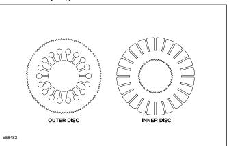
The sun shaft has male splines that connect to the viscous coupling inner hub; the outer viscous coupling is driven by the annulus via four drive pegs. The viscous action only occurs when there is a relative speed difference at the front and rear drive wheels due to reduced traction on either axle.
