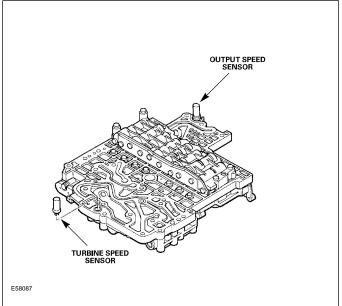
Both speed sensors are inductive pulse generators, which provide the TCM with a transmission speed alternating voltage signal. The pickup (coil) portion of the sensors are mounted to the valve body; the reluctors are integrated with transmission rotating components. The TSS sensor reluctor has 30 teeth; the OSS sensor reluctor has 36 teeth.
