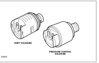
Shift solenoids SSM1, 2 and 3 are used to shift the transmission through all forward gears and reverse. They are two-way on / off normally closed solenoids. The TCM controls the solenoids by switching the ground side of the circuit.
