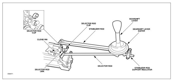
In order to isolate the outer gearshift mechanism from the bodywork, the gearshift housing is located in a remote gearshift mounting that is rigidly joined to the transmission by the gearshift stabilizer. This mounting can move lengthways to balance the rotational movements of the engine/transmission.
