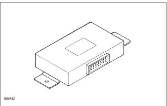
Actual transmission control changes are made by actuators (solenoids) that respond to driver outputs provided by the TCM. These solenoids operate in response to electrical signals; they regulate the control valve operation. The control valves cause changes in the fluid flow passages. These changes result in pressure changes within the transmission.
