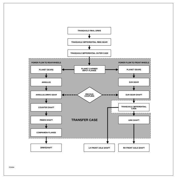
The 40% / 60% torque split is achieved by the ratio of radius to gear tooth contact on the annulus and sun gears, where they contact the planet gears, as indicated by the arrows shown in the diagram.
