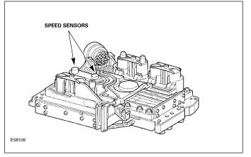
The pickup (coil) portion of the sensors share a common molded platform and mount to the valve body electrical module. The reluctors are impulse rings that are attached to transmission rotating components. To ensure that the correct distance is maintained between the pickups and the impulse rings, the sensors are held in position by a leaf spring that rests against the valve body. The speed sensors are serviceable only as a unit. **Speed Sensors**
