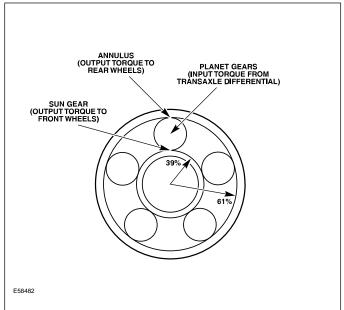
Under normal driving conditions, all the components of the center differential rotate at the same speed, with front and rear torque split determined by the lever ratio of the tooth contacts. **Viscous Coupling Discs**
