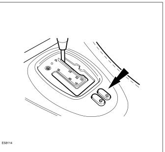
The W5A580 transmission system has two available Reverse gear ratios. When Normal is selected, the TCM implements the Reverse ratio; when Sport is selected, the TCM implements the Low Reverse ratio.
