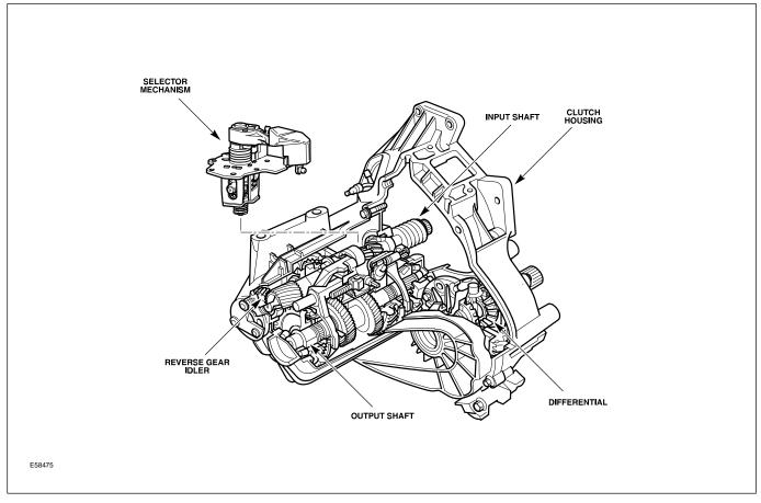
To further improve stability and gear shifting, a maintenance-free cable operating mechanism is used. All the gear wheels, including reverse gear, are helical cut, synchronized, and run on needle roller bearings. First, second, and third gear have double synchronization. The advantages of double synchronization are that the transmission runs quietly, gearshifts are smooth, and the assembly is compact and light in weight.
