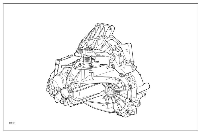
The MTX-75 is a two-shaft design, with all pairs of gears in continuous mesh. Each forward gear ratio is produced through a single pair of dedicated gears, with
