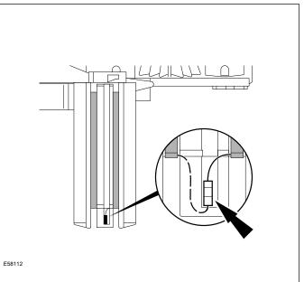
**NOTE:** The TFT sensor is in a series circuit incorporating a Park and Neutral reed switch. The switch is not used for transmission control, and monitoring of transmission fluid temperature is limited to when D or R is selected only. If the selector is in P or N, engine coolant temperature is substituted.
