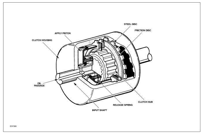
Pressurized oil acts on the apply piston moving the piston in contact with the clutch pack. The hydraulic pressure forces the discs together and the resulting friction connects the discs causing the housing and hub to rotate (or hold) together as one unit. When the hydraulic pressure is released, the clutch return springs move the apply piston away from the clutch discs, allowing them to once again rotate freely.
