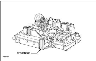
Transmission fluid temperature is determined by the TCM by the change in the sensor resistance. The TCM applies 5 volts (nominal) to the sensor and monitors the voltage across the pins to detect the varying resistance. TFT is one of the main factors used by the TCM to calculate shift and pressure control. If the TFT sensor signal is lost, the TCM will substitute engine coolant temperature (CAN message).
