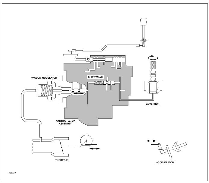
Modulator Valve and Governor (Conventionally Controlled Transmissions)
