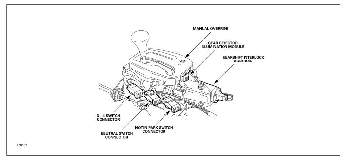
The J-gate assembly incorporates three micro switches:
