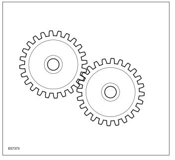
The input and output torque will be the same; therefore, the torque ratio is also 1:1.
