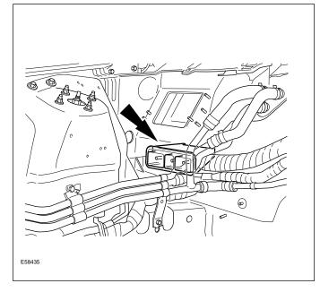
**Powertrain Control Module Connector Faces**
