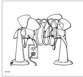
drive member is called the pump impeller and is in turn driven by the engine. The driven member is called the turbine and in turn drives the transmission input shaft. As the torque converter rotates, its shape gives acceleration to the fluid.
