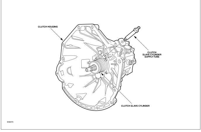
The central slave cylinder is fixed to the clutch housing with four bolts, together with an integrated release bearing press-fit on the clutch slave cylinder.
