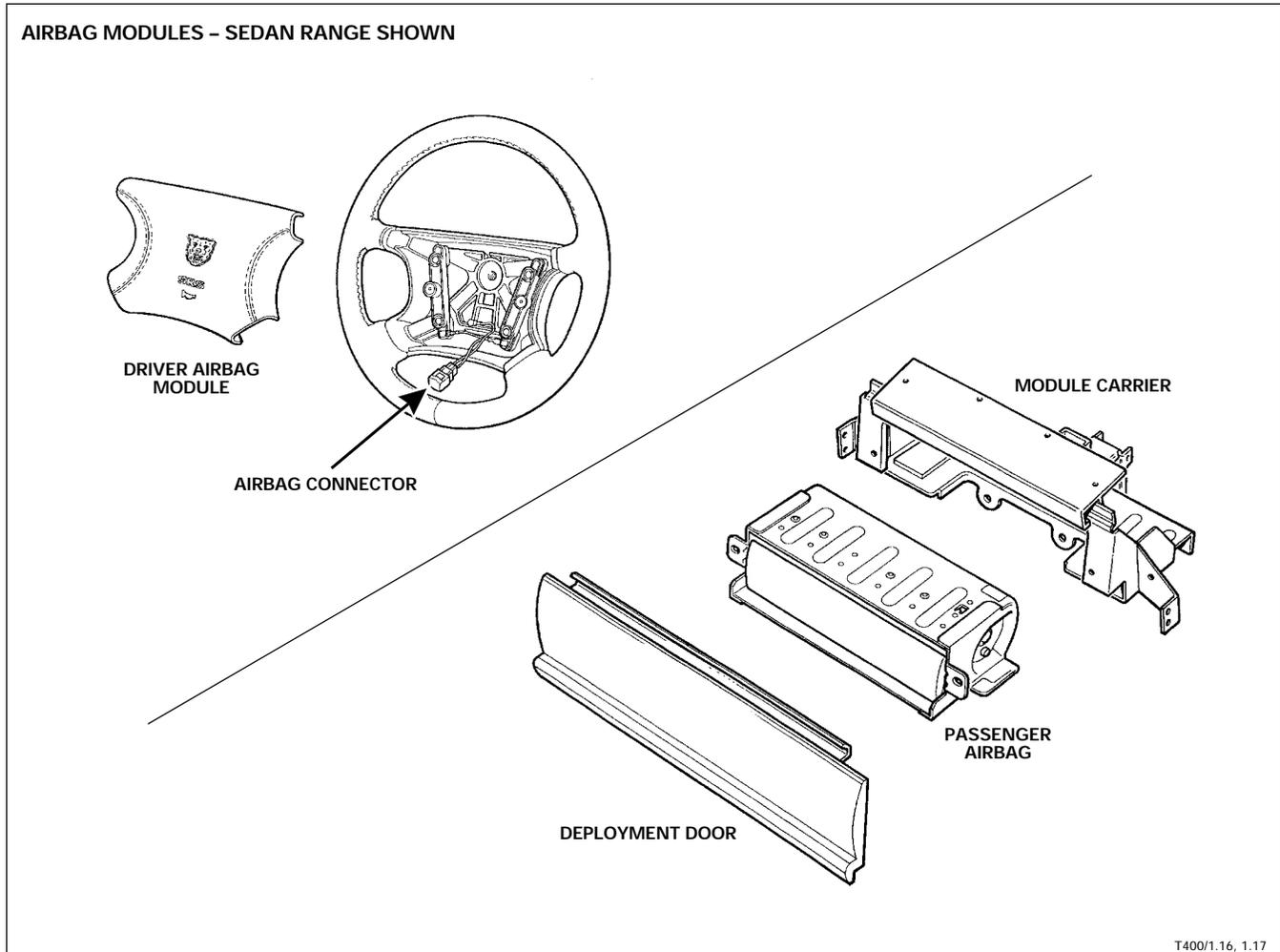
When the safing sensor plus one impact sensor is activated (contacts closed), the circuit from the DM deployment voltage supply (or reserve voltage supply) is completed through the safing sensor to each airbag and to ground at the activated impact sensor (or dwell enhancer). Current flow triggers the igniter, which in turn ignites the deployment charge. The time from sensor closing to airbag deployment is no greater than 32 milliseconds.
