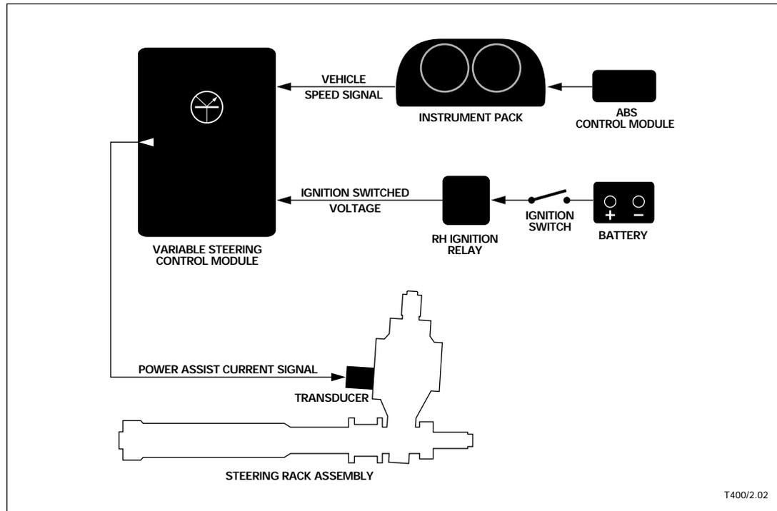
**Variable steering control module diagnostic monitoring**
