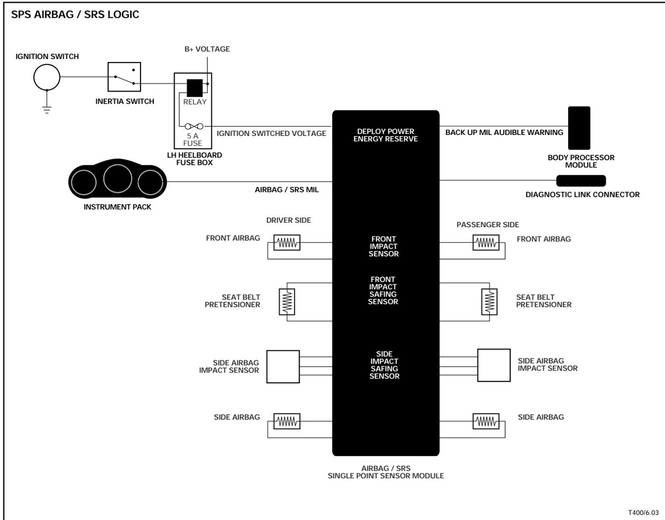
The front airbags, seat belt pretensioning retractors, side impact sensors, and side airbags are connected to and powered by the SPS. The SPS receives power from an ignition switched 5 A fused supply via the left hand heelboard fuse box.
