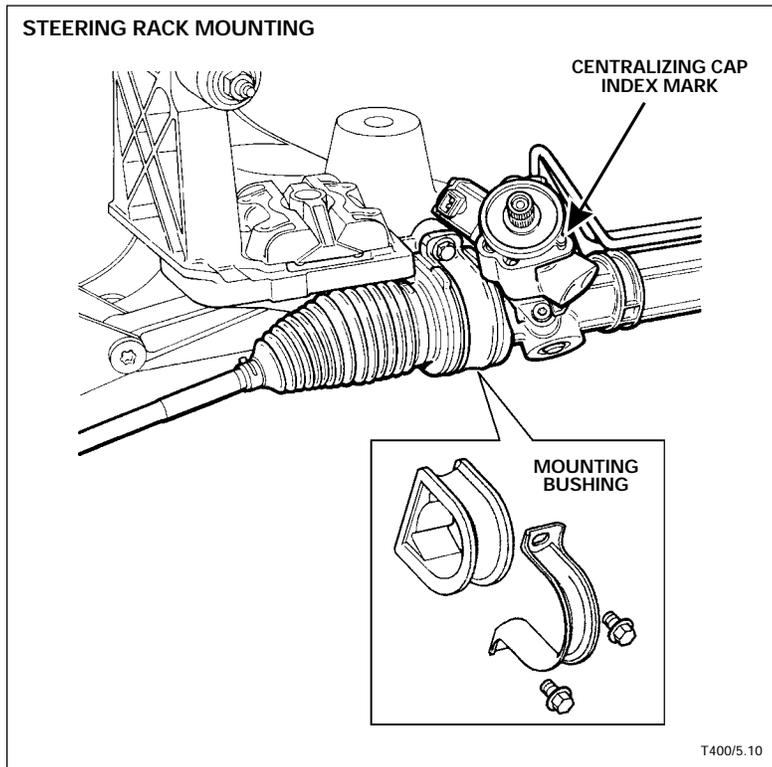
The steering rack assembly is mounted directly to the subframe in rubber bushings. Because of its variable ratio design, the steering must be centered during steering column or suspension geometry adjustment. To center the steering, align the pinion centralizing cap with the index mark on the pinion / valve assembly.
