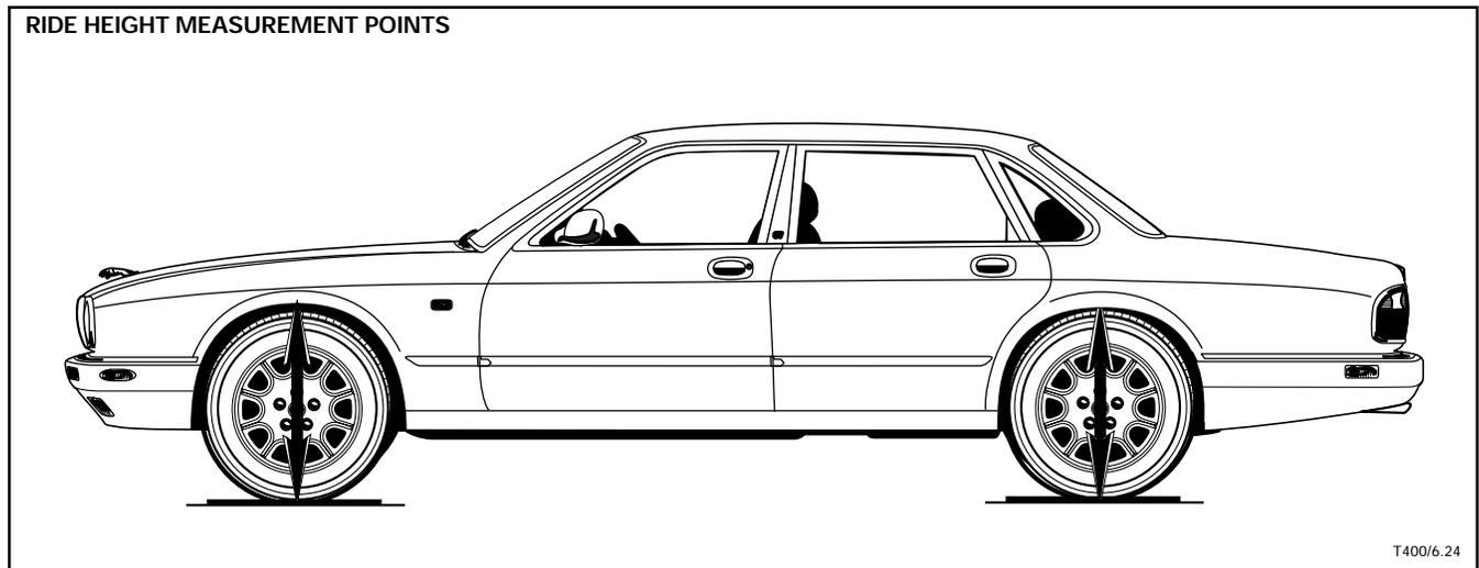
Ride height is measured from the alignment equipment slip plates to the top of the wheel arch.
