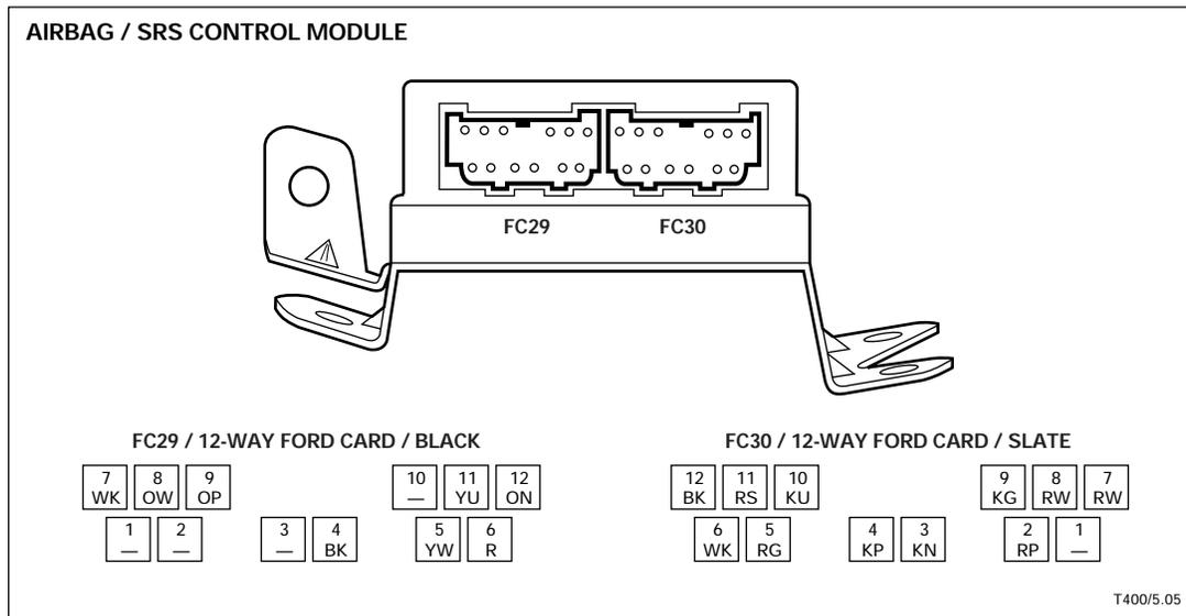
**Airbag / SRS control module pin out information**
