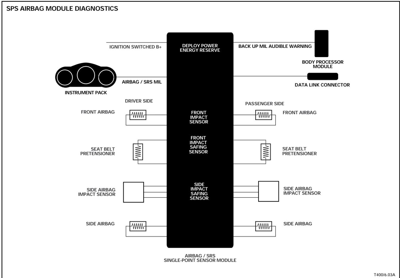
The SPS module logs all system DTCs including the time, in running hours, that the fault occurred. If a fault is intermittent, the MIL is activated and the DTC logged with the time, in running hours, that the fault occurred and the time that the fault was corrected. The MIL remains active until the ignition is switched off. If the fault is not present when the ignition is next switched on, the MIL is not activated. However, the DTC and its time of occurrence remains in SPS memory.
