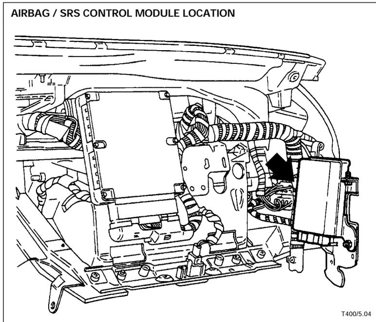
**Airbag / SRS Control Module**
