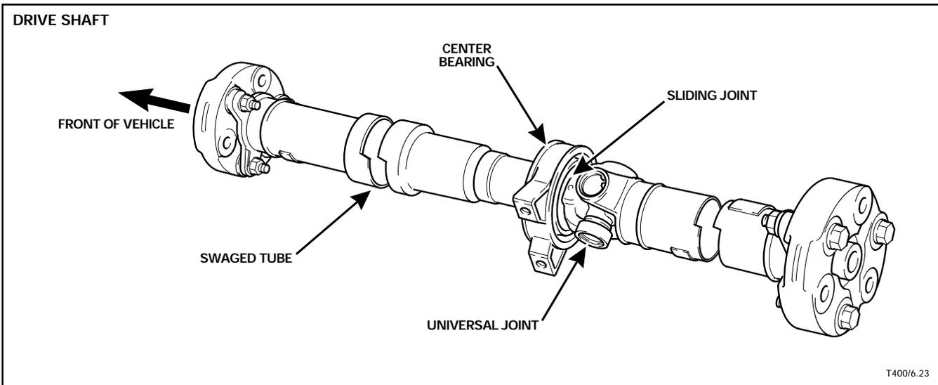
The front half of the drive shaft is manufactured with a swaged tube section to provide collapse in the event of a collision. The front and rear halves are connected at the center bearing with a splined sliding joint. The center universal joint is relocated to the rear half of the drive shaft. Flexible couplings connect the assembly to the transmission and final drive flanges.
