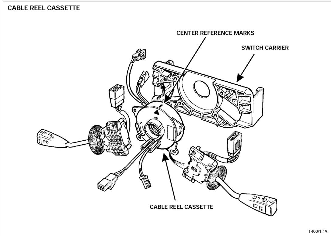
When installing the cassette, center the steering and align the cassette center reference marks to provide for steering wheel rotation without damage to airbag circuit wiring.
