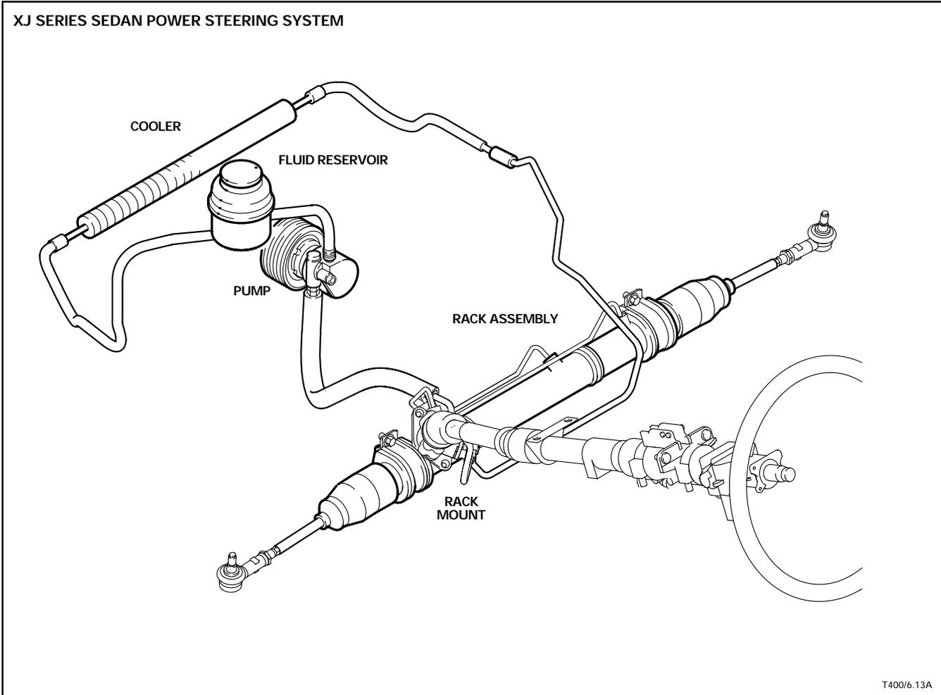
**Steering Reservoir, Pump, and Fluid Cooler**
