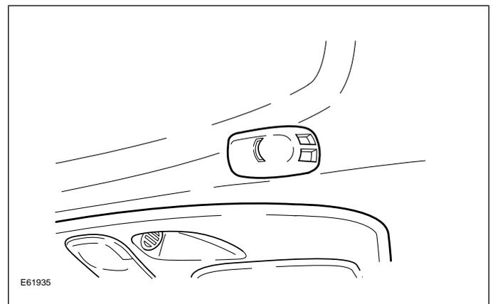
There are two types of microphones used on Jaguar vehicles. The V60 factory fit microphone is integrated into the overhead console. For dealer installation, the microphone is located above the driver and is attached to the headliner. It is also recommended that this microphone be installed when V60 systems are upgraded to Bluetooth, as the the external microphone has improved clarity versus the factory microphone.
