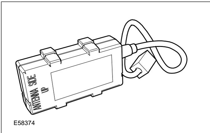
The BTUM has one electrical connector and communicates with the PSE module by it's own proprietary communications bus.
