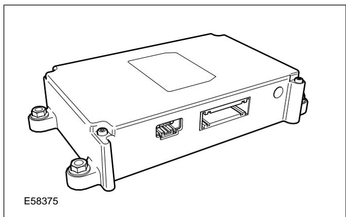
For all X200, X300 and X400 series vehicles, the PSE module is fixed in a bracket which also supports the Voice Activation Control Module (VACM) and the navigation control module. If the PSE module is being
