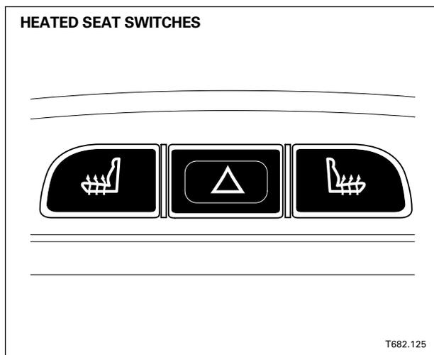
Pressing the appropriate switch facilitates the three-stage operation of the heated seat function:
