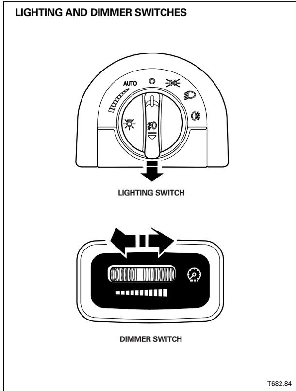
The instrument pack will illuminate with Sidelights ON. Instrument pack decodes the position of the dimmer switch and the lighting switch, and then broadcasting *SCP – BACKLIGHTING INTENSITY AND DIMMING CURVE WITH HEADLAMPS COMMAND* to the following:
