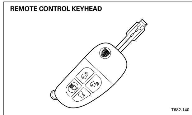
The Radio frequency (RF) operation is suspended 22 days after the last valid RF signal is received. This is reactivated by the change of state of any of the latch switches (for example, door ajar, lock / unlock, and so on.). After 22 days the customer can not use any RF feature until the RF operation is reactivated.
