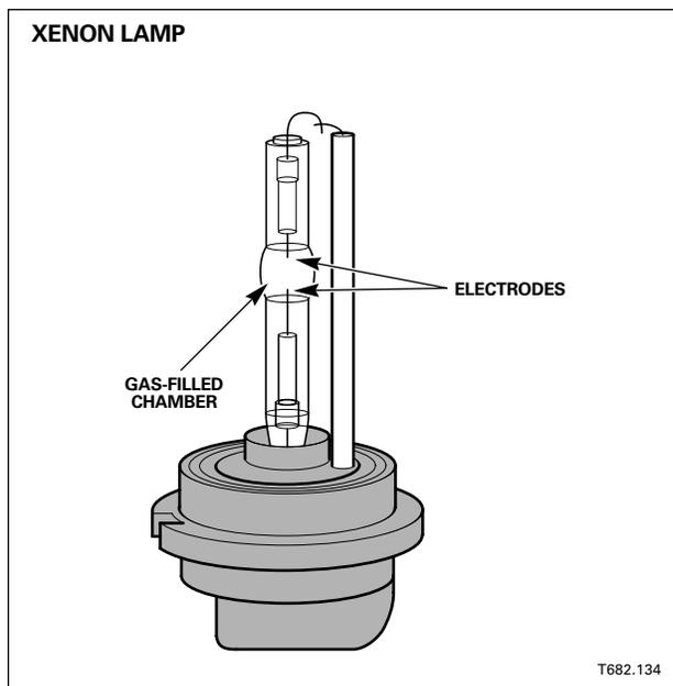
The 35-watt xenon lamp produces a beam with an intensity that is approximately two times that produced by a halogen lamp of the same wattage. The chamber of the bulb contains xenon gas and a mixture of metal halide salts.
