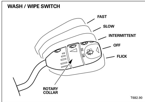
The wash / wipe system is entirely hardwire controlled and activated. All of the driver controlled inputs are to the GECM from the column stalk switch. The GECM directly activates the wash / wipe components.
