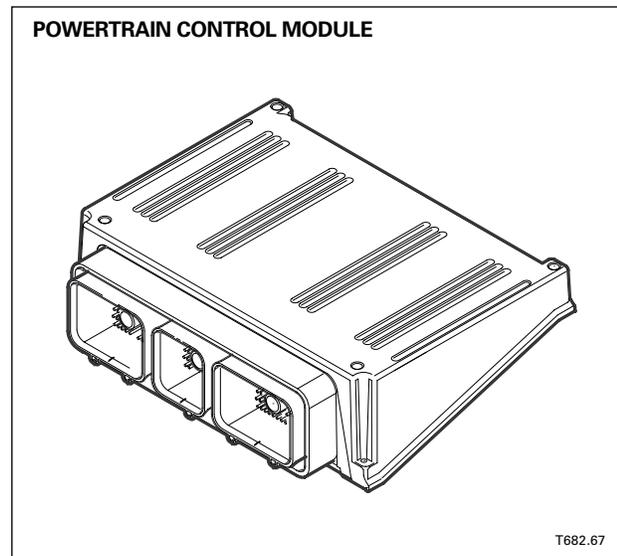
**NOTE:** The PCM must be configured to the instrument pack as part of the security system set up. If this is not carried out, the engine will not start. Refer to “Instrument Pack” on page 4.2.6.
