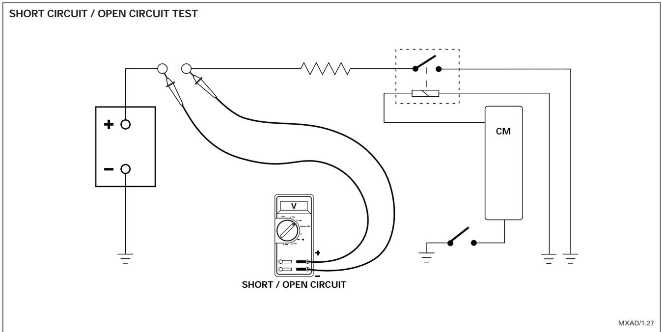
If there is a voltage reading, there is a short circuit before the circuit control components.
