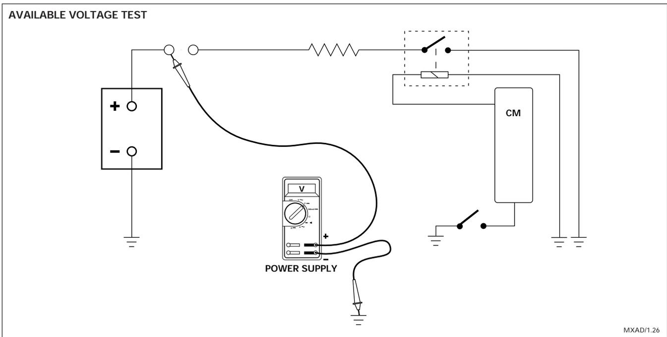
If there is no voltage or low voltage, the power supply is insufficient. (ALWAYS CHECK THE POWER SUPPLY).
