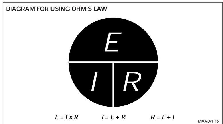
For example, if the electrical potential ( $E$ ) and the current ( $I$ ) are known, but the resistance ( $R$ ) is not, divide the electrical potential ( $E$ ) by the electrical current ( $I$ ) to find the electrical resistance ( $R$ ):  $R$  (ohms) =  $E$  (volts)  $\div$   $I$  (amperes).
