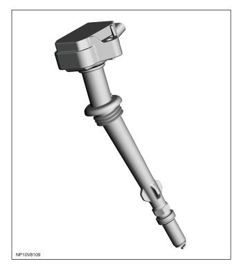
Energy is stored in the primary winding's magnetic field by allowing a current to flow through the primary circuit switched by the switching module.
