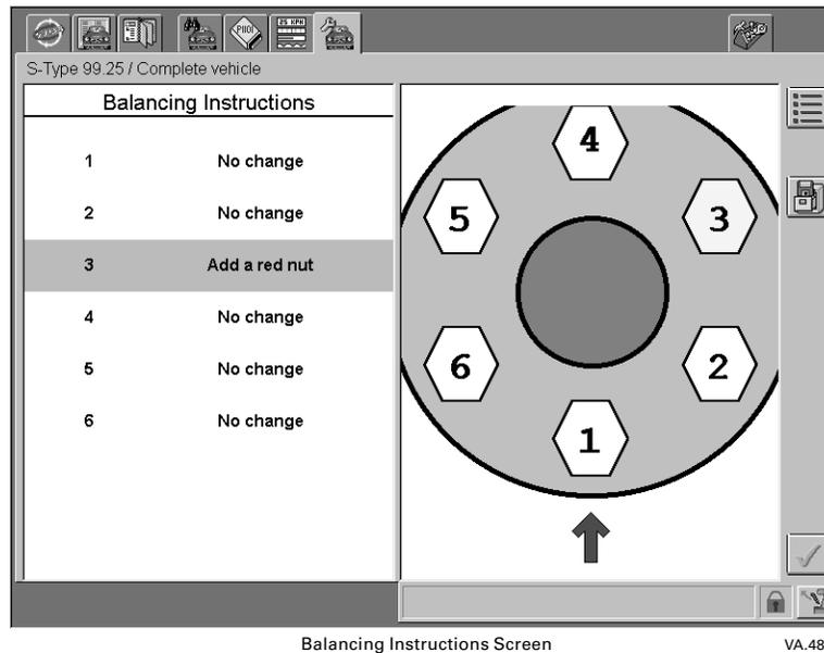
At the conclusion of a successful capture session the PTU displays a comprehensive diagnostic report. Fit the appropriate weighted nut to the bolt as instructed to correct the imbalance, then carry out a second capture event to verify the imbalance has reduced or disappeared.
